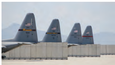
A response to IDF activity. “T-Walls” emplaced to protect C-130s at Bagram. (Reproduced by permission from John A. Tirpak, “The Aerial Life-line,” Air Force Magazine 95, no. 8 [August 2012], http://www.airforce.mag.com/MagazineArchive/Pages/2012/August%202012/0812life-line.aspx .)
