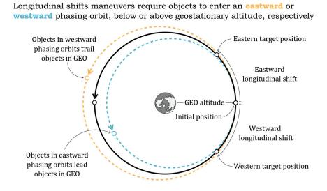
Figure 2: Nominal eastward and westward longitudinal shift maneuver orbits in GEO
