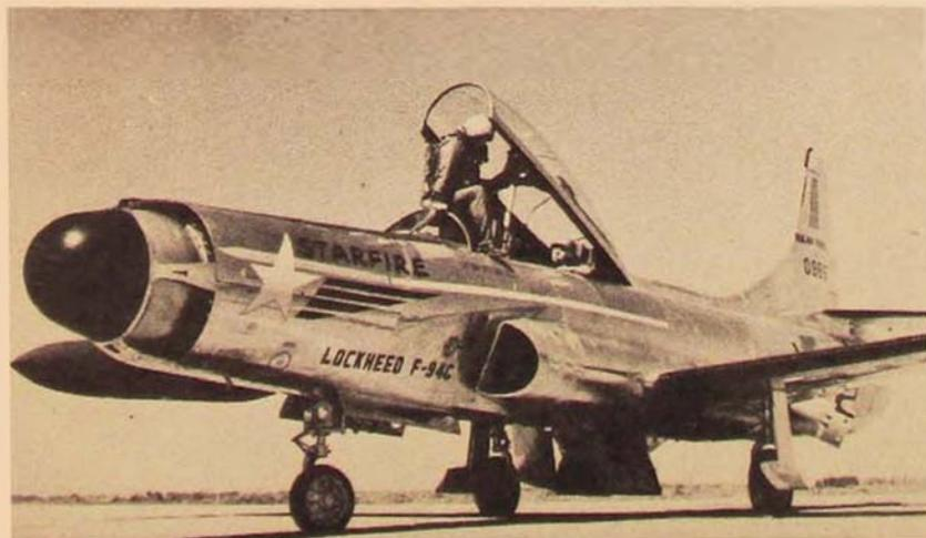
*consists of 24, 2.75-inch rockets which are ranged, aimed, and fired electronically from the ring of tubes around the black-domed radar nose. The rocket doors are closed in flight, snap open before firing. Wing rockets, 1,000-pound bombs, or napalm tanks can be attached under the thin, sturdy wings.*
