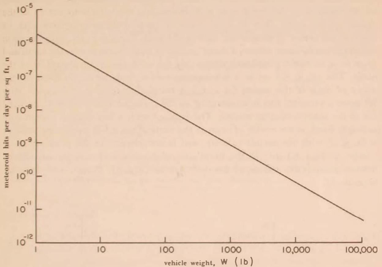
Figure 3. Frequency of hits by meteoroids that will impart a velocity of 0.1 ft/sec or more to the vehicle.
