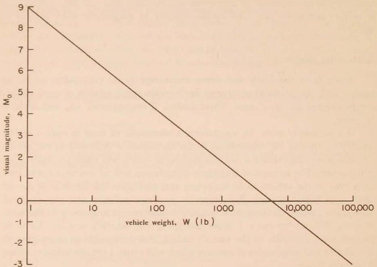
Figure 2. Limiting magnitude of meteoroids that will impart a velocity of 0.1 ft/sec or more to the vehicle.
