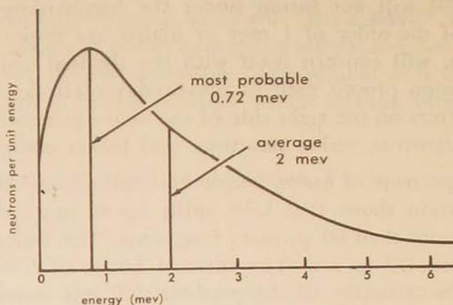
Figure 1. Neutron fission energy spectrum.
