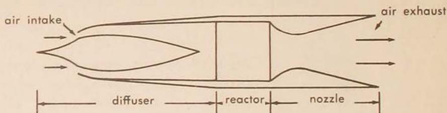
Figure 1. Basic elements of a nuclear-ramjet "engine."
