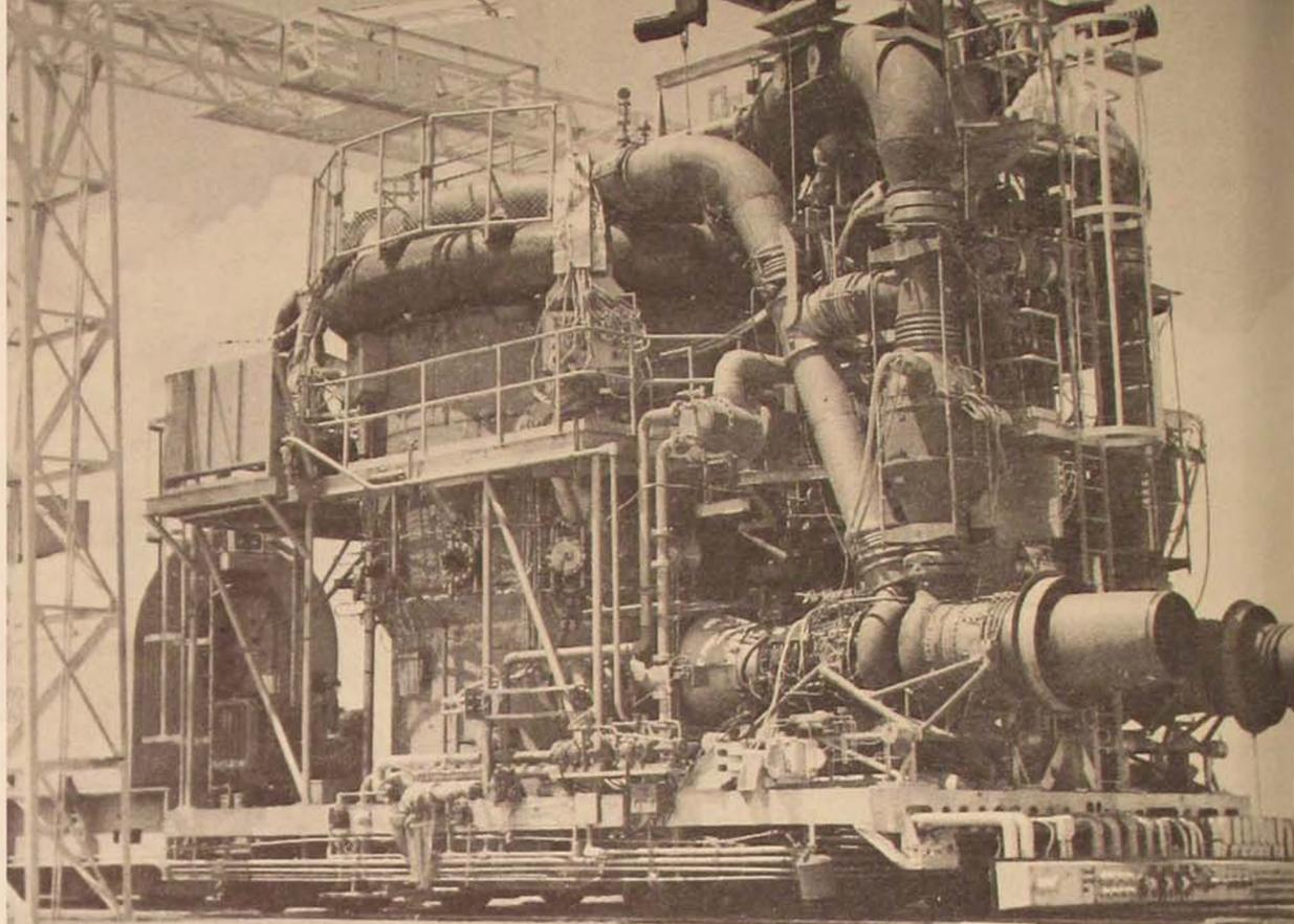
*Figure 4. Core Test Facility at the Idaho Test Station, NRTS, showing the developmental assembly for HTRE-1 with its two turbojet engines protruding at the right.*
