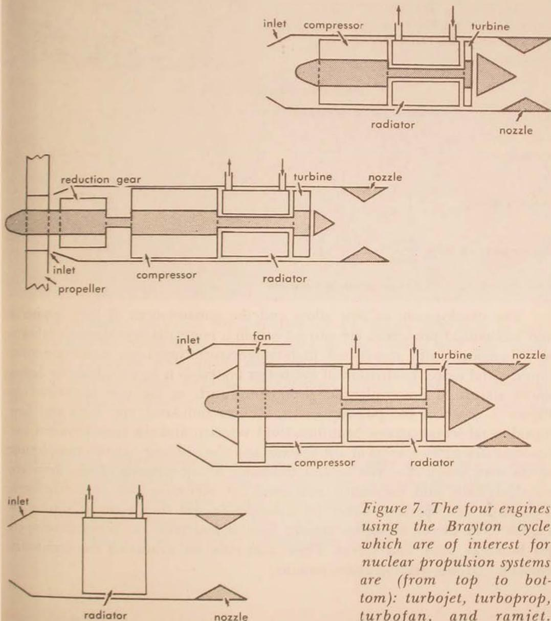
Figure 7. The four engines using the Brayton cycle which are of interest for nuclear propulsion systems are (from top to bottom): turbojet, turboprop, turbofan, and ramjet.
