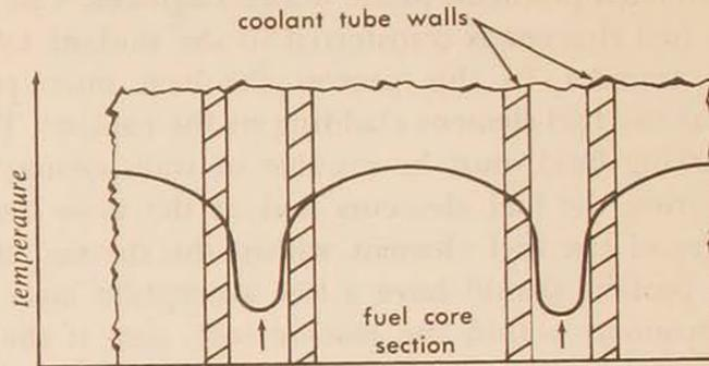
Figure 2. Temperature profile across coolant channels.
