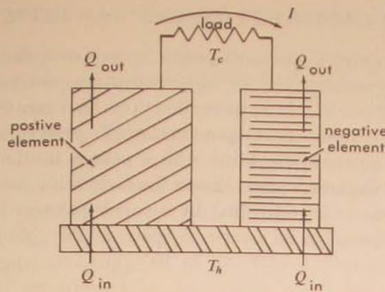
Figure 1. Thermoelectric conversion device.
