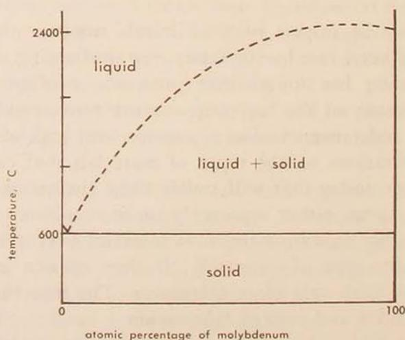
Figure 1. Formation of plutonium-molybdenum phase (a metallic fuel and metal alloy). A bimetal system in which each of the metals is completely soluble in the other admits selection of an alloy in any desired proportion of the two metals.
