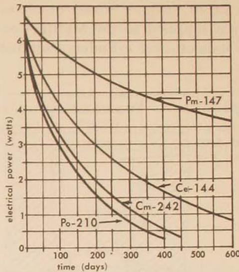
Figure 4. Isotope electrical power versus time.
