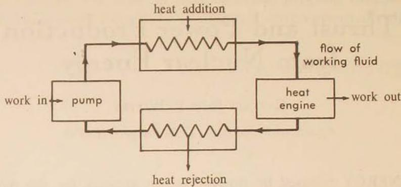
Figure 1. Basic thermodynamic cycle (the direct-cycle, closed-cycle system).
