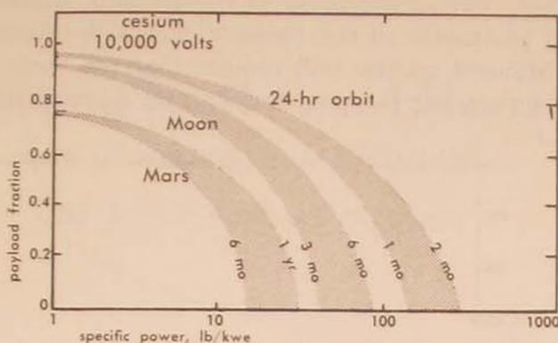
Figure 9. Assumed nuclear-generated electric propulsion requirements and payload capabilities for space missions to Mars and the moon and for a 24-hour orbit.
