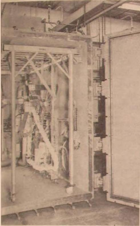
*Figure 9. Forced-convection, liquid-metal corrosion loop, triangular shaped, installed in inert-atmosphere chamber.*
