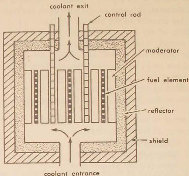
Figure 2. Schematic of heterogeneous thermal reactor.
