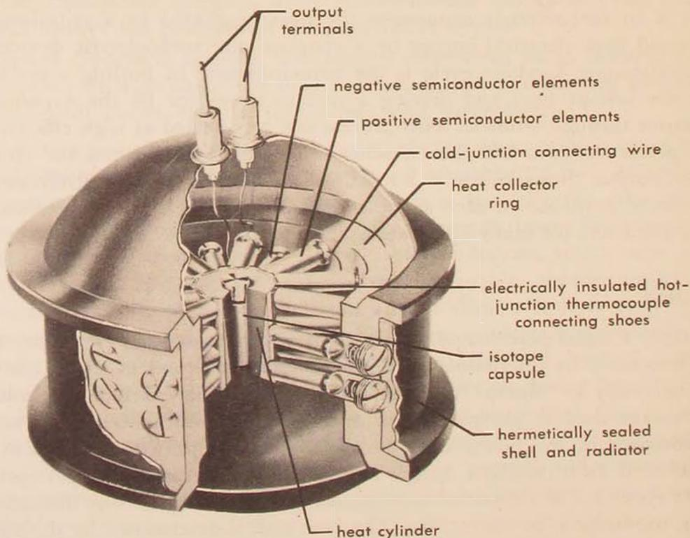
Figure 2. Snap-3, cutaway diagram.
