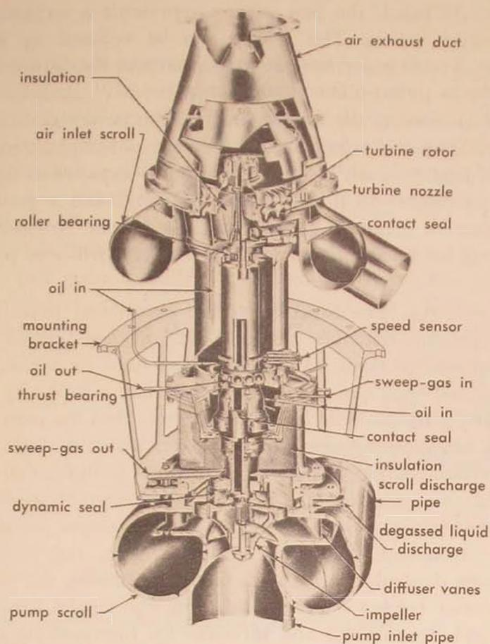
Figure 6. Liquid-metal turbopump TP-1.
