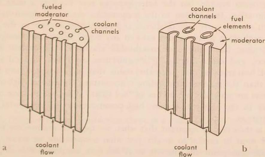
Figure 1. Two types of reactor cores: (a) half section of a solid, homogeneous core showing the coolant channels through the core; (b) half section of a heterogeneous core having hollow-rod fuel elements through which the coolant flows.
