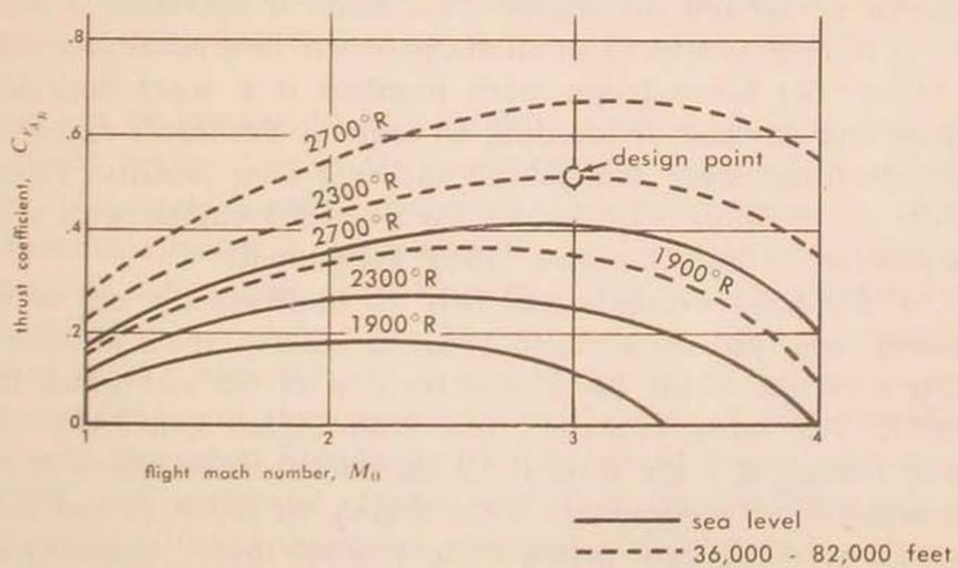
Figure 5. Nuclear-ramjet thrust coefficients of Figure 4 based on reactor frontal area instead of free-stream capture area, for flights at sea level and at 36,089 to 82,000 ft altitudes. The six temperatures shown are reactor temperatures.
