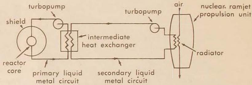
Figure 3. Two-loop, liquid-metal, indirect-cycle propulsion system.
