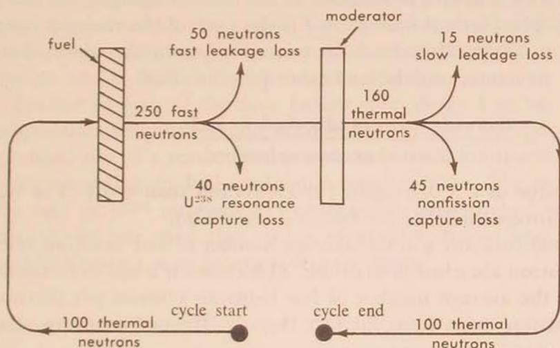
Figure 3. The self-sustaining chain criticality.
