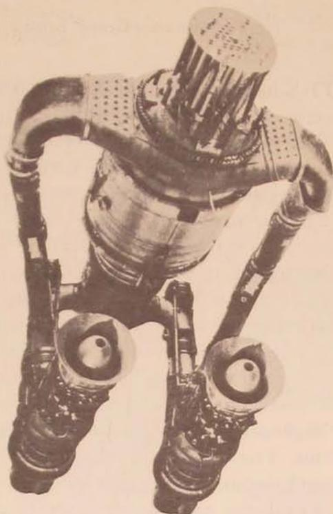
*Figure 7. HTRE-3, showing essential components of the system—the reactor and the two jet engines.*
