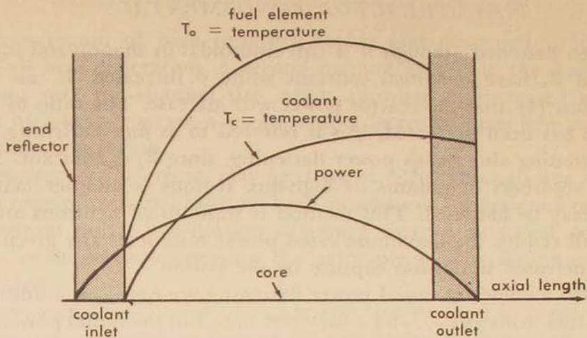
Figure 7. Axial distributions in a heterogeneous cylinder.
