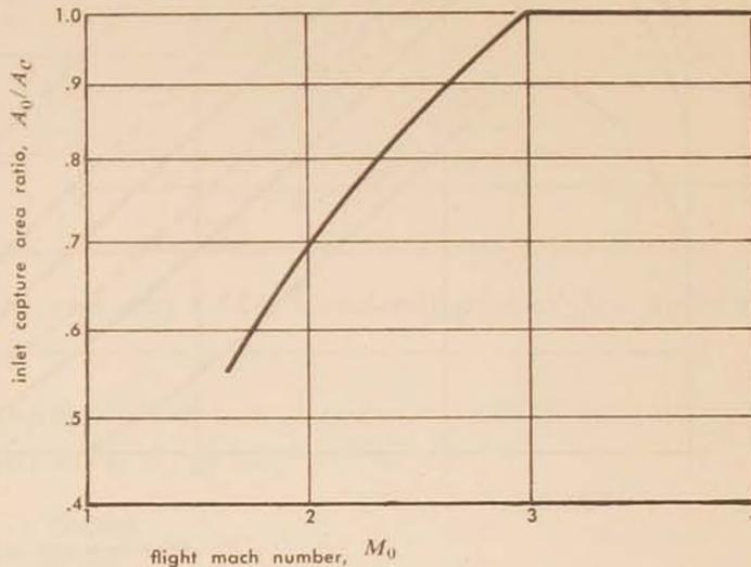
Figure 6. Curve showing the assumed inlet airflow (or inlet-capture-area ratio) versus the mach number for a 30° conical inlet designed for mach-3 operation.
