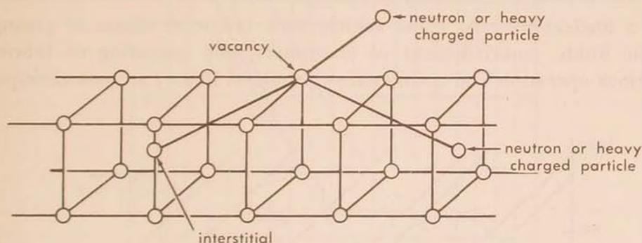
Figure 4. The Frenkel defect—displacement of atoms in the lattice structure.
