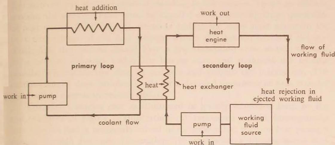
Figure 3. Indirect-cycle system.
