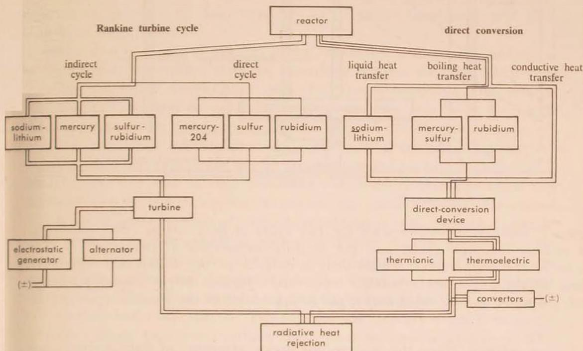
Figure 6. Advanced nuclear auxiliary-power-unit systems.
