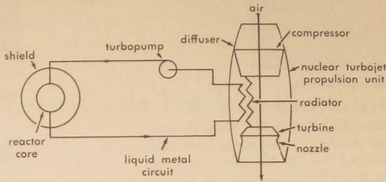
Figure 2. Single-loop, liquid-metal, indirect-cycle propulsion system.
