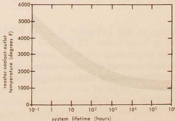
Figure 5. System lifetime versus operating temperatures.
