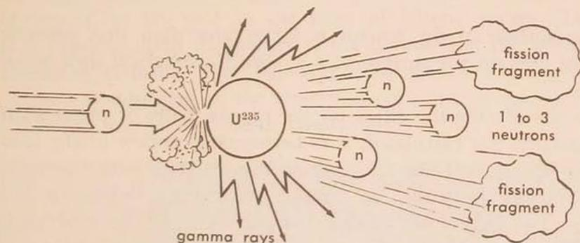
Figure 1. The fission reaction of uranium-235.
