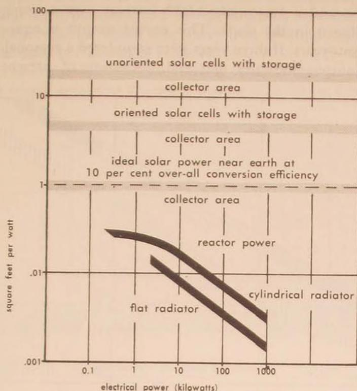
Figure 1. Radiator-area and collector-area requirements for satellite APUs.
