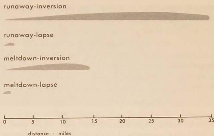
Figure 1. Extent of 1-MPE hazard after selected types of accidents.
