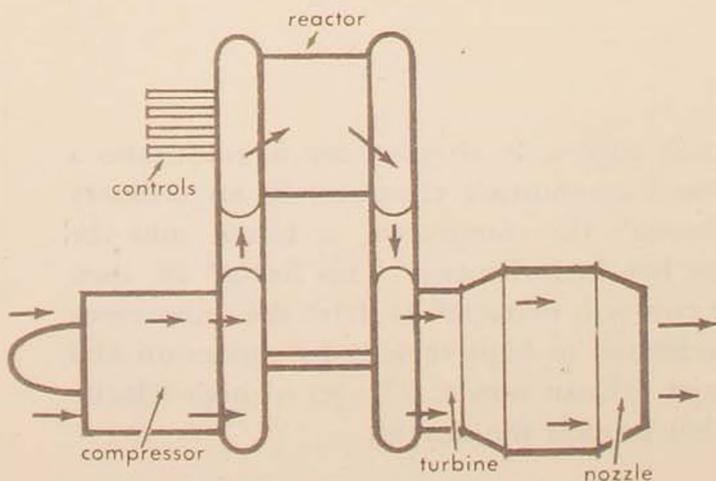
*Figure 2. Schematic of direct-air-cycle nuclear propulsion system. Air enters through the compressor, is forced into the reactor, and heated by the fuel elements. After passing through the turbine, where energy is extracted to drive the compressor, the heated air is expelled at high velocity through the exhaust nozzle.*
