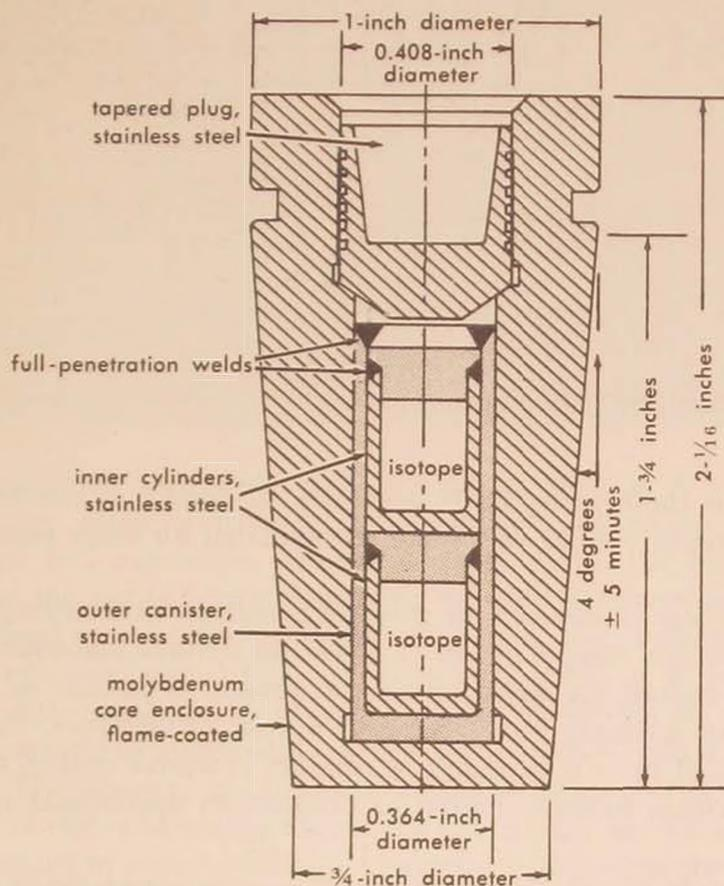
Figure 3. Internal containment of radioisotope in Snap-3.
