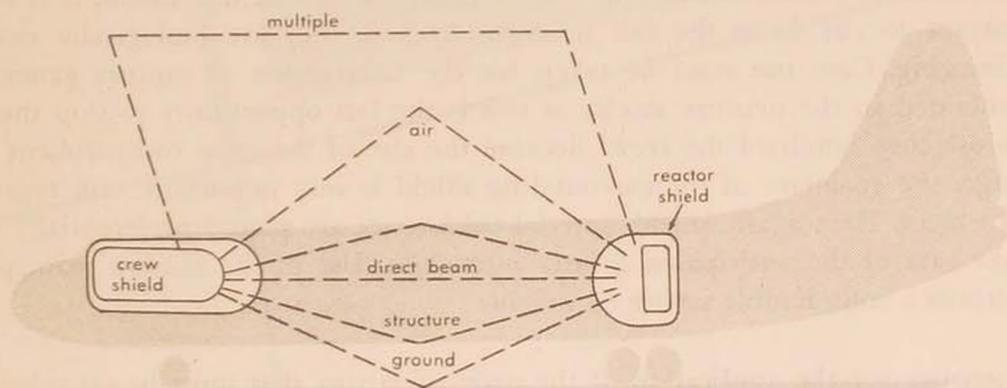
Figure 9. The effect of air, ground, and aircraft structure in redirecting scattered radiation from the nuclear reactor toward the crew compartment shield.
