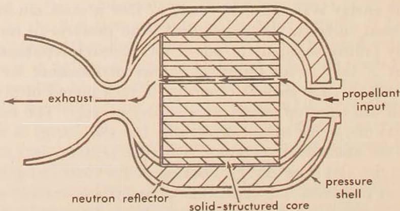
*Figure 1. Schematic diagram of the solid-fuel heat-exchanger propulsion reactor. Propellant is pumped through a number of parallel channels in the reactor core and removes heat generated in the nuclear fuel plates. It then expands through a convergent-divergent nozzle to exert thrust by virtue of its momentum. Not shown here are the control rods, methods of support, methods of cooling the pressure shell, or the nozzle—all of which are essential to an actual propulsion reactor.*
