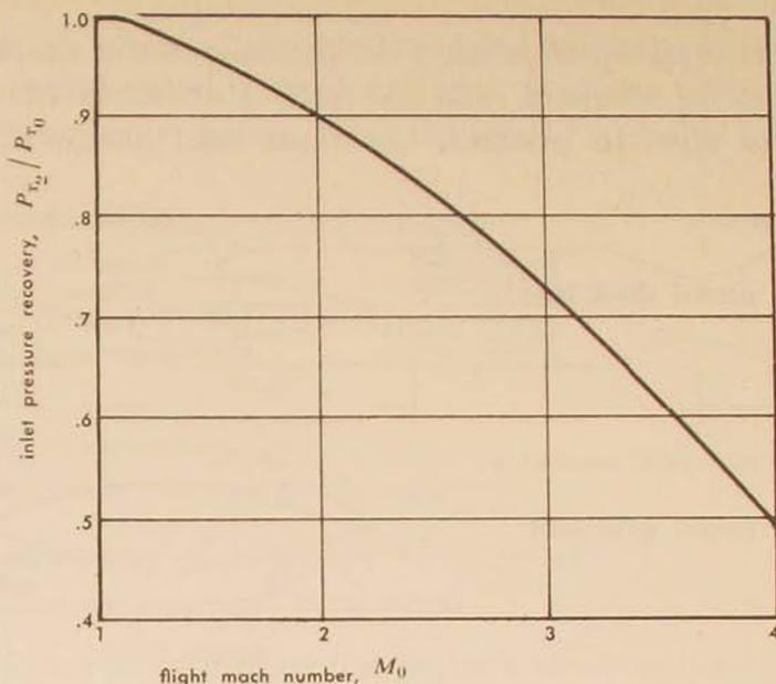
Figure 3. Inlet pressure recovery (AIA standard) plotted for flight mach number.
