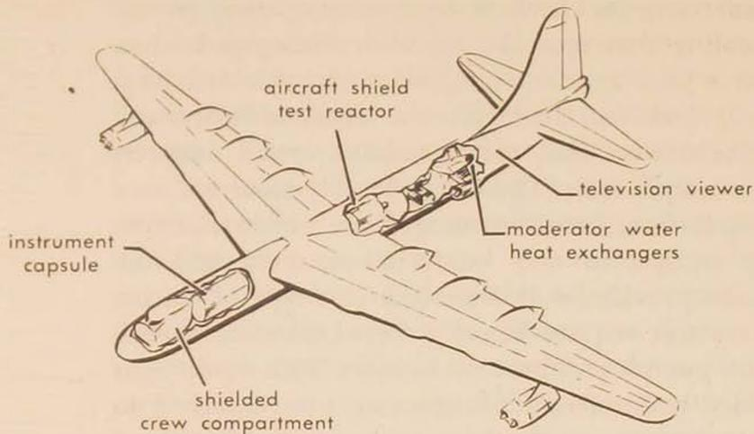
*Figure 1. Nuclear Test Aircraft flights permitted study of shielding, radiation effects on the aircraft, and methods of flight and ground operations. Diagram identifies special equipment of the NTA.*
