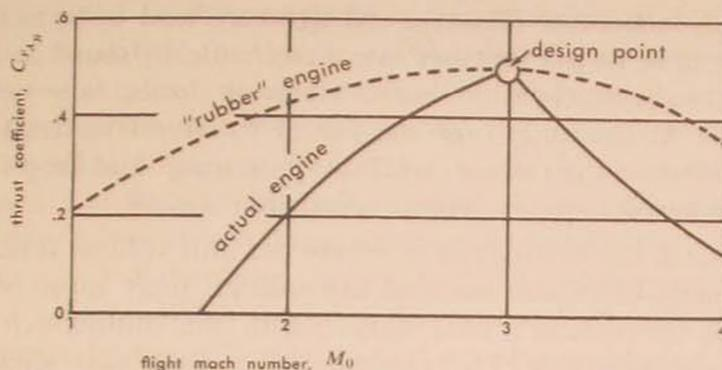
Figure 7. Off-design performance of a mach-3 engine with a reactor outlet temperature of  $2300^{\circ}\text{R}$ , and comparative rubberized performance data from Figure 5.
