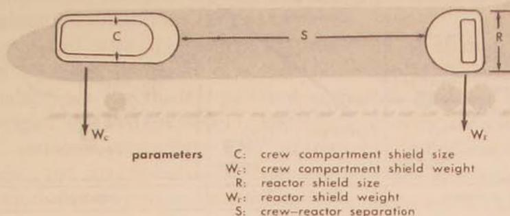
Figure 7. Divided-shield parameters affecting aircraft design.
