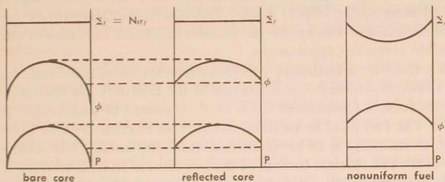
Figure 6. Fuel, flux, and power radial distribution.
