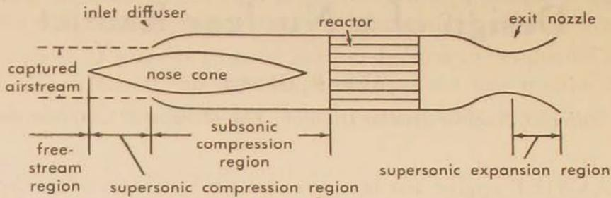
Figure 1. Simplified schematic of a nuclear-ramjet engine.
