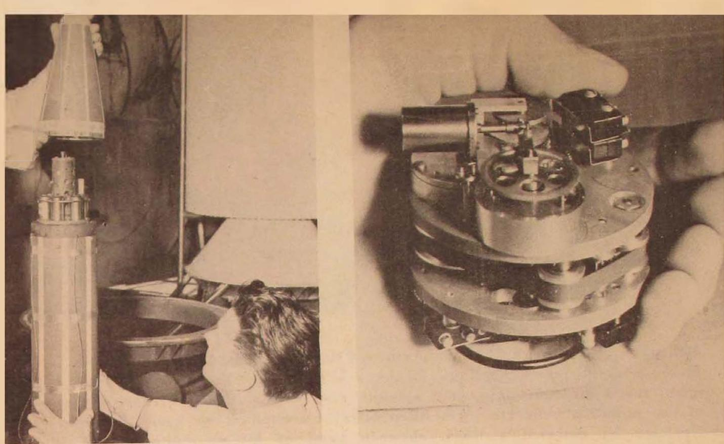
*Protective nose cone (left) is lowered over Explorer III's instrumentation, which included a miniature tape recorder (right). Explorer III (cutaway below) transmitted data on temperature, cosmic-dust erosion, and intensity of cosmic radiation.*
