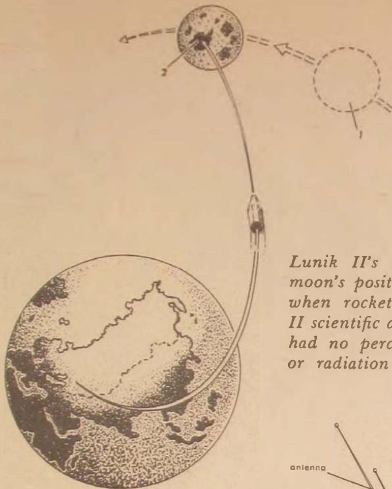
*Lunik II's trajectory (left) shows moon's position at launch (1) and when rocket impacted (2). Lunik II scientific data revealed the moon had no perceptible magnetic field or radiation belts surrounding it.*
