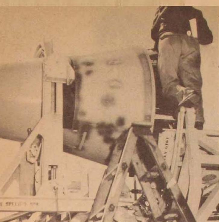
*Before and after views of mating the nose cone (containing the re-entry vehicle) to the Discoverer satellite. The cloth cover helps maintain prelaunch temperature.*
