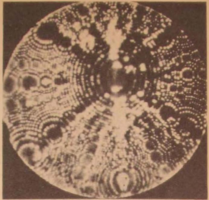
*Figure 2. Photographs of a single atom on the tip of a tungsten needle. Taken by a field emission microscope, the photo at left is magnified 4,300,000 times, the one on the right 2,750,000 times.*
