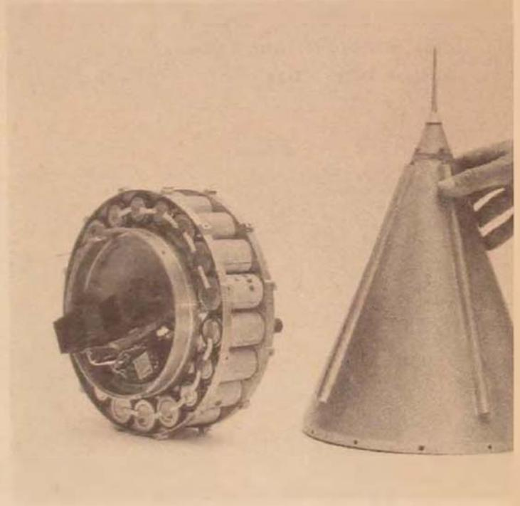
*Pioneer III's radiation deck (left) has two Geiger-Mueller tubes and a voltage supply tube. An underside view (right) shows the photoelectric scanning device and batteries for radio beacon and cosmic-ray experiment. The cone, gold-washed for electric conductivity, serves as antenna. Pioneer III is shown in cutaway above.*
