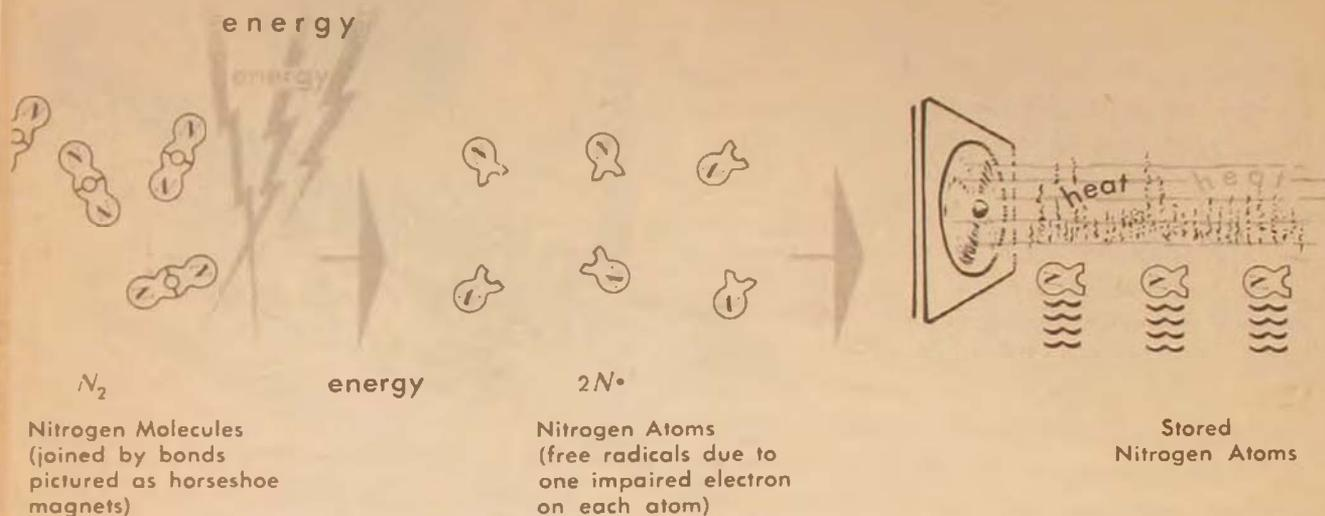
Figure 11. The free-radical process. In the formation and storage phase, shown in (a), nitrogen molecules—or many other varieties—are energized to the point that the bonds tying the molecules together are broken. This frees nitrogen atoms (free radicals), which can then be solidified by removal of heat. In the recombination
