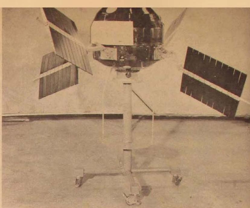
*Explorer VI, the paddle-wheel satellite, is unique in two respects: its four solar paddles, and its TV scanner to take the first crude pictures of the earth from space. The paddles are in launching position (left), orbiting position (right).*
