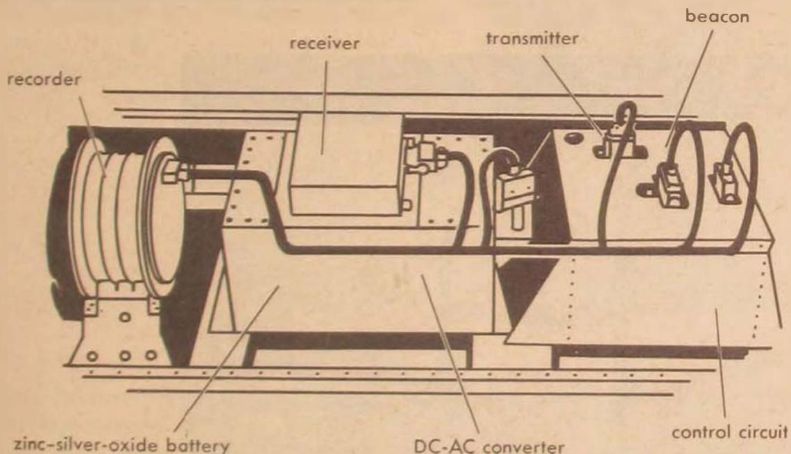
*Cutaway diagram of one of the twin communications relay systems carried in Project Score Atlas satellite to receive, store, and relay messages from ground stations.*
