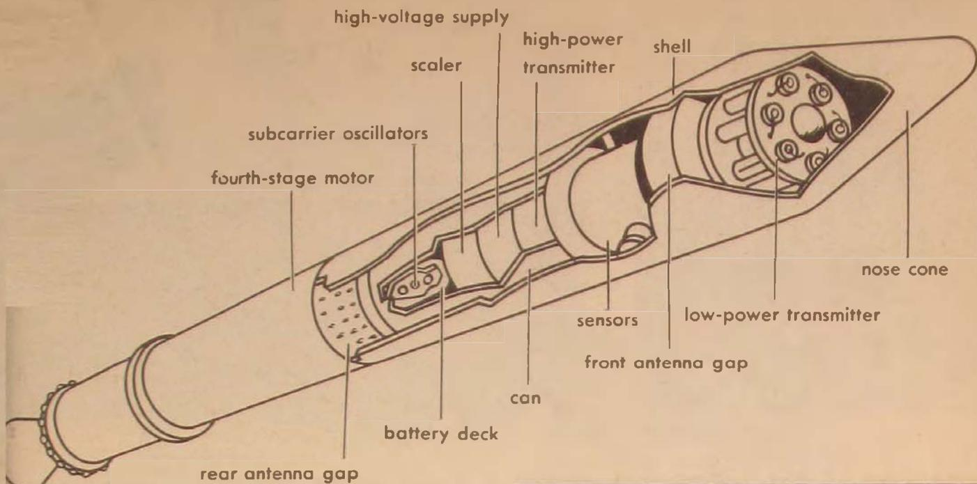
*Explorer IV, shown in cutaway above, is installed on a Jupiter-C rocket. It was designed and instrumented to investigate high corpuscular radiation intensities detected by Explorers I and III.*
