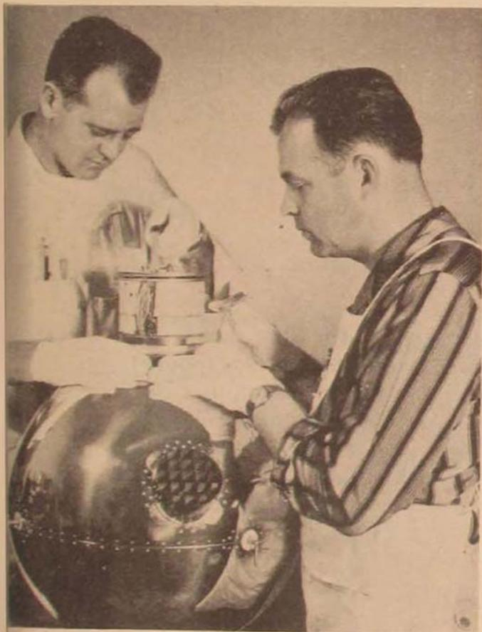
*Vanguard II satellite: cutaway (above); instrument-deck insertion (left); atop launching rocket.*
