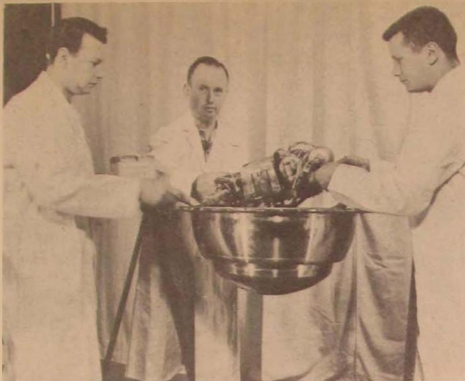
*The environmental capsule is placed in Discoverer II's re-entry capsule (top). At right is a rear view of the completely assembled re-entry capsule, containing a parachute.*
