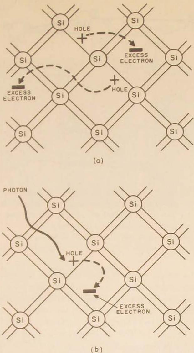
Figure 3. Covalent bonds broken by thermal vibrations (a) and by photon (b)
