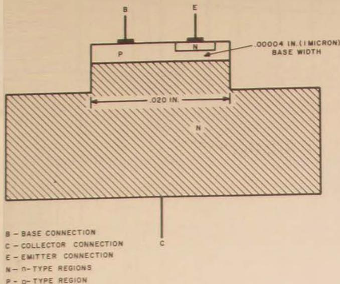
Figure 15. Cross-section view of a mesa transistor (not drawn to scale)
