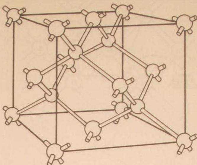
Figure 2. The diamond lattice structure. Atomic lattice for the diamond form of carbon and the semiconductors silicon, germanium, and gray tin. Covalent electrons are shared between each pair of nearest-neighbor atoms.
