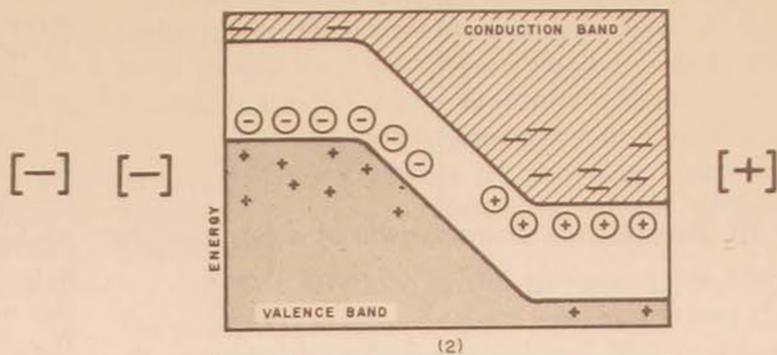
Figure 9a. Dipole layer and p-n junction with forward voltage applied, showing decrease in dipole layer with forward voltage (1), and p-n junction decreased by forward voltage (2)
