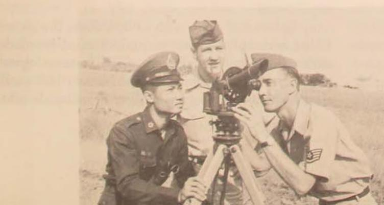
*... and track a weather balloon by using a theodolite.*
