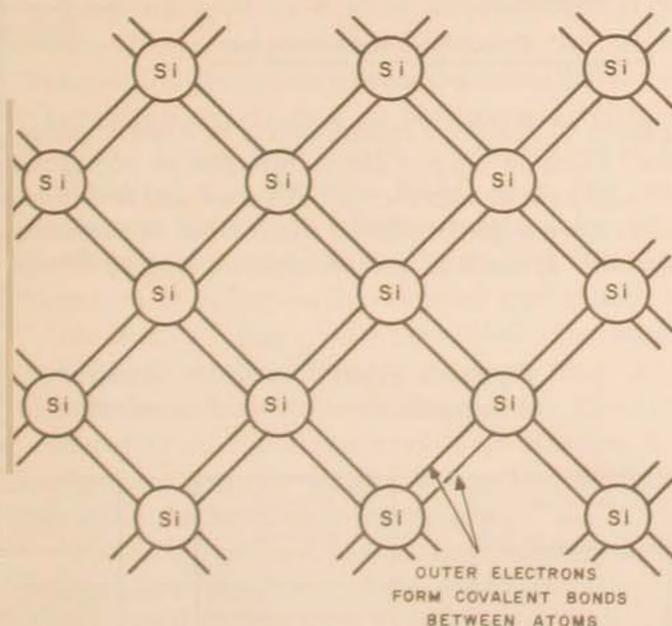
Figure 1. Silicon atom and covalent bonding. Silicon atom (a), showing four outer electrons. Each silicon atom shares covalent bonds with its four nearest-neighbor atoms (b).
