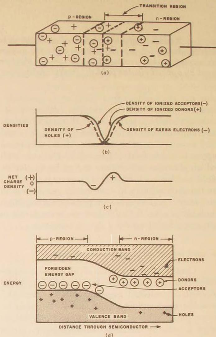
Figure 8. The *p-n* junction, showing semiconductor containing *p-n* junction (a); densities of impurities and charge carriers (b); net charge density, giving dipole layer (c); and energy level diagram for the *p-n* junction (d)
