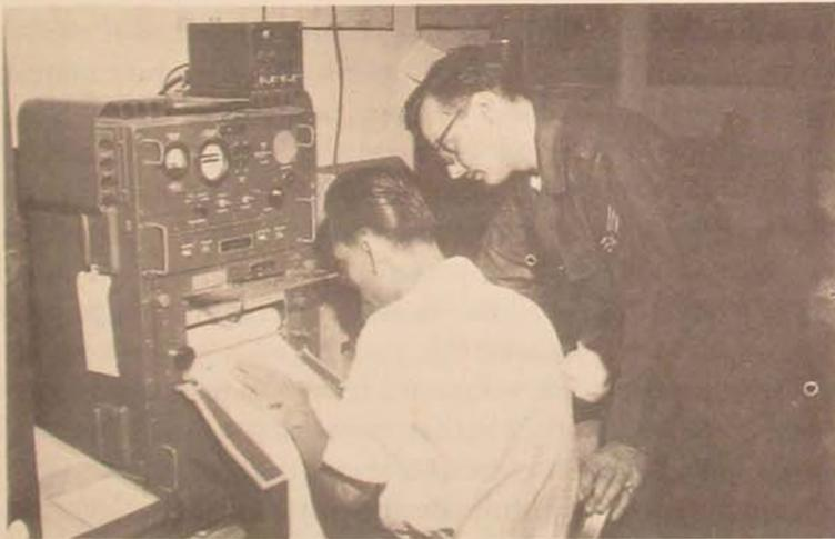
*... check the signal strength of rawinsonde on this radar-like receiver—*
