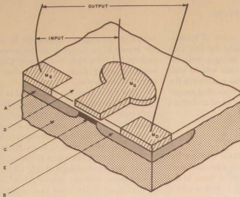
Figure 17. Section through a metal-oxide-silicon transistor
