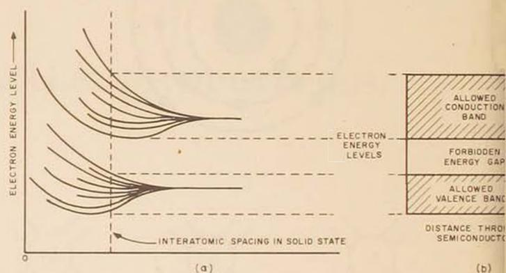
Figure 4. Electron energy levels in a semiconductor. Electron energy levels broaden as atoms are brought closer together (a). Allowed and forbidden electron energy bands (b) result from the splitting up and spreading out of electron energy levels.
