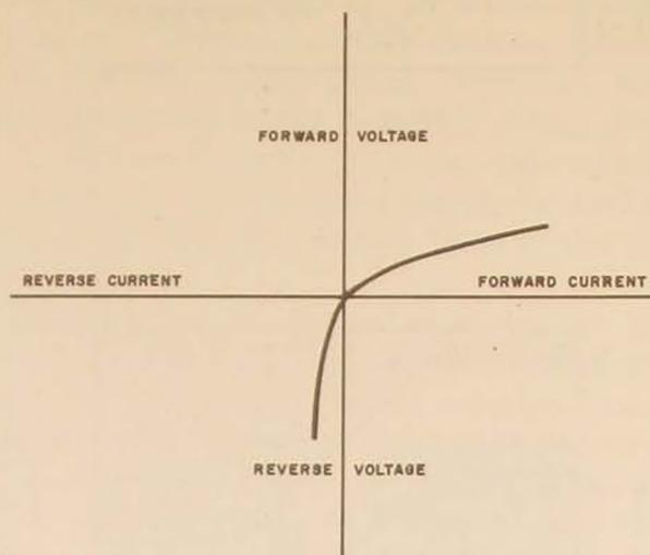
Figure 10. Rectification characteristic of a p-n junction
