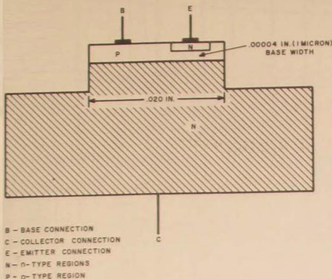
Figure 15. Cross-section view of a mesa transistor (not drawn to scale)
