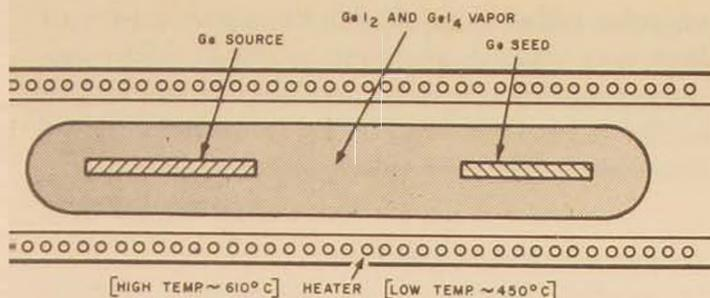
Figure 13. Closed-tube method of vapor growth of germanium
