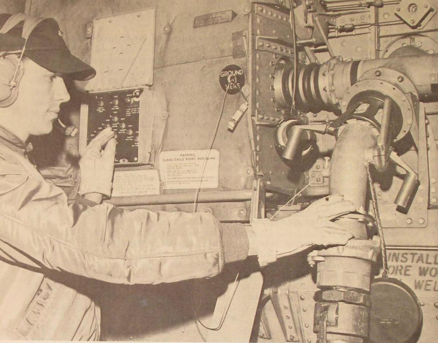
*Plugged in and flowing. Through this single pipe, a MATS transport can take on a full load of fuel from 50,000-gallon bladders lying in the open field. No longer do maintenance men have to drive big tank trucks up to the aircraft and clamber over the wing.*
