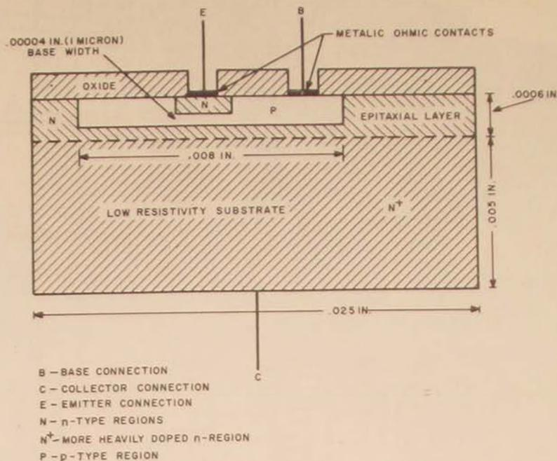
Figure 16. Cross-section view of a planar transistor (not drawn to scale)
