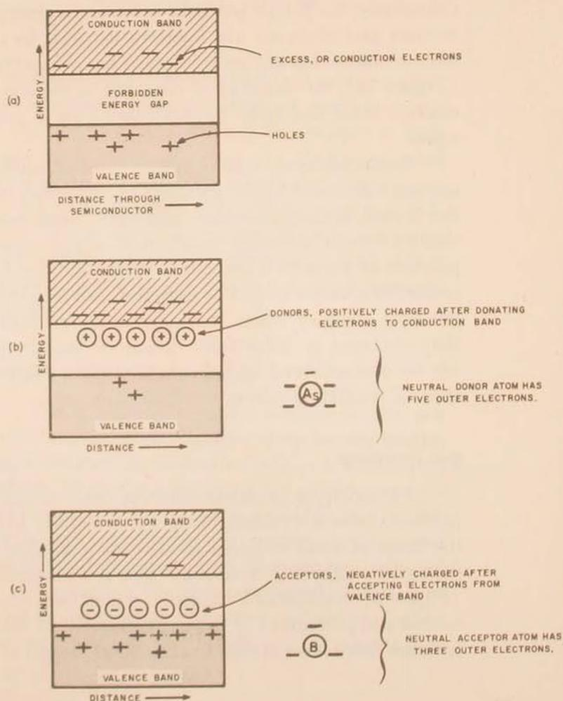
Figure 7. Excess electrons and holes in intrinsic semiconductor (a), in n-type semiconductor (b), and in p-type semiconductor (c)
