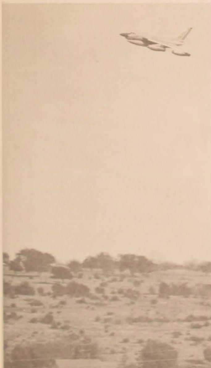
*Most B-58 training missions have at least one leg of low-level flying. The delta wing gives the B-58 an unusually smooth low-altitude ride at speeds just under the speed of sound. All supersonic flight is at altitudes above 30,000 feet. A B-58 (below) touches down after a training mission. Drag-chute deceleration saves brakes and tires.*
