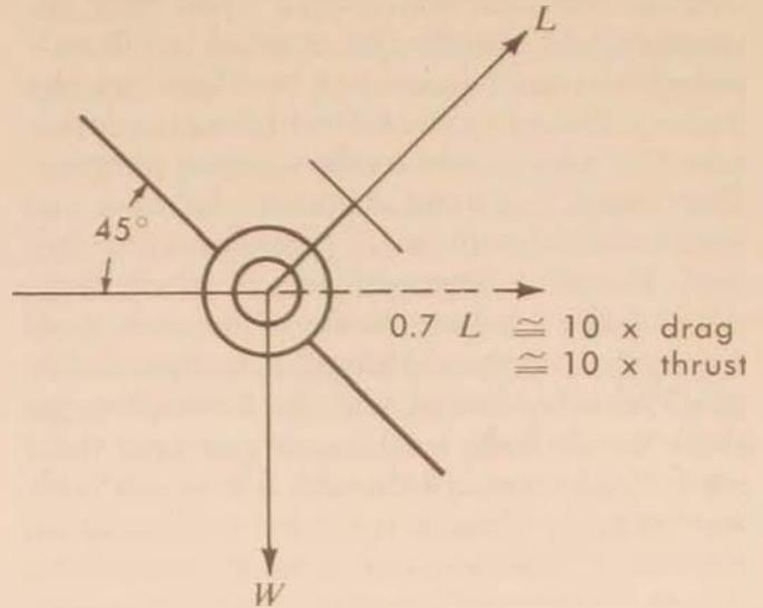
Figure 2. Forces on an aircraft in a horizontal turn
