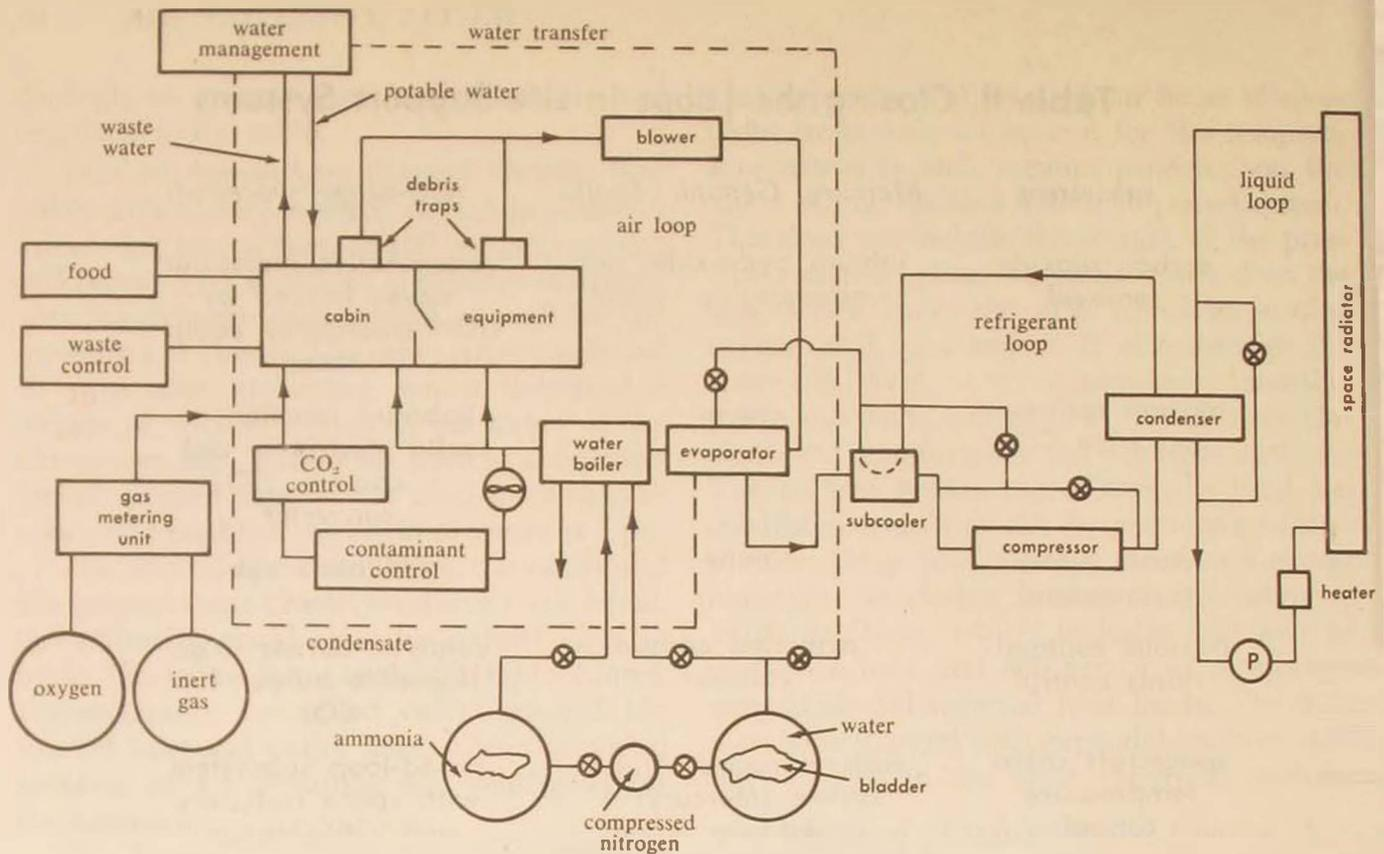
Figure 2. Active thermal and atmospheric control system, cabin and equipment in parallel
