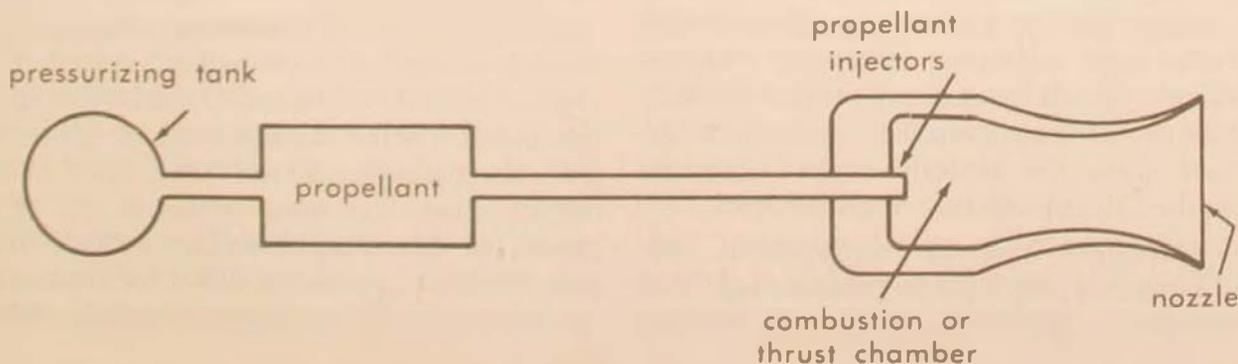
have been previously combined in the proper proportions in the main propellant tank, mixing at the injector is not required. The propellant is ignited in the combustion chamber, and the exhaust products are forced rearward out the nozzle, providing the desired thrust.
