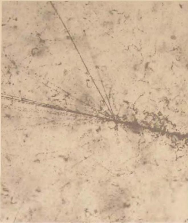
*The simplest and most economical way to measure high-energy particles is by photo emulsion techniques. When a high-energy particle strikes an atom in the emulsion materials, the number and density of "star" prongs produced denotes energy of the particle.*
