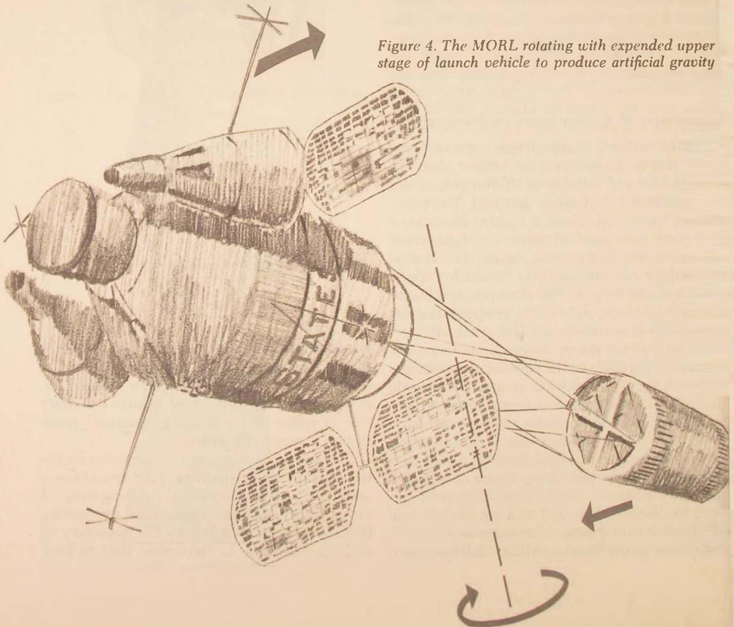
Figure 4. The MORL rotating with expended upper stage of launch vehicle to produce artificial gravity
