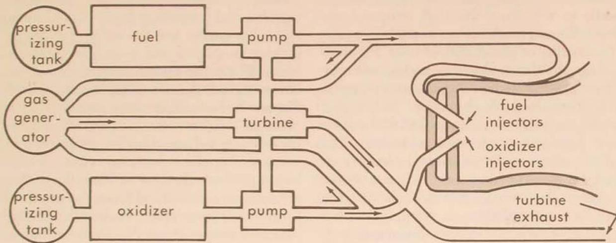
Figure 8. Schematic of pump-fed liquid bipropellant (bootstrap) system
