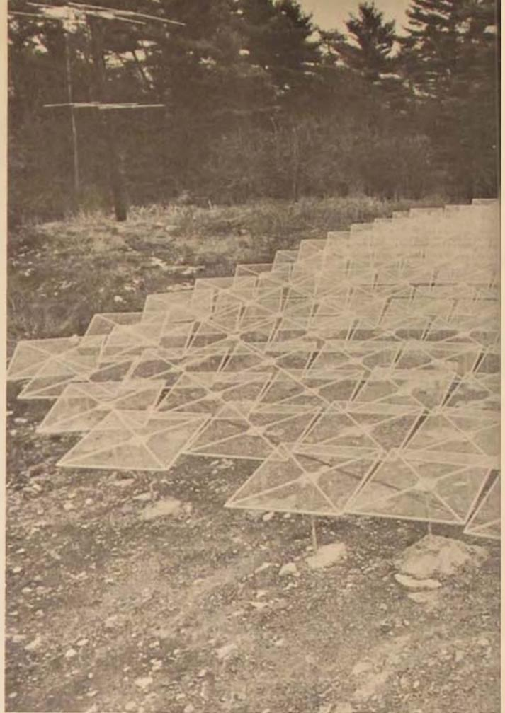
*This experimental model of the multiplate antenna was located at Concord, Massachusetts. Initial the-*
