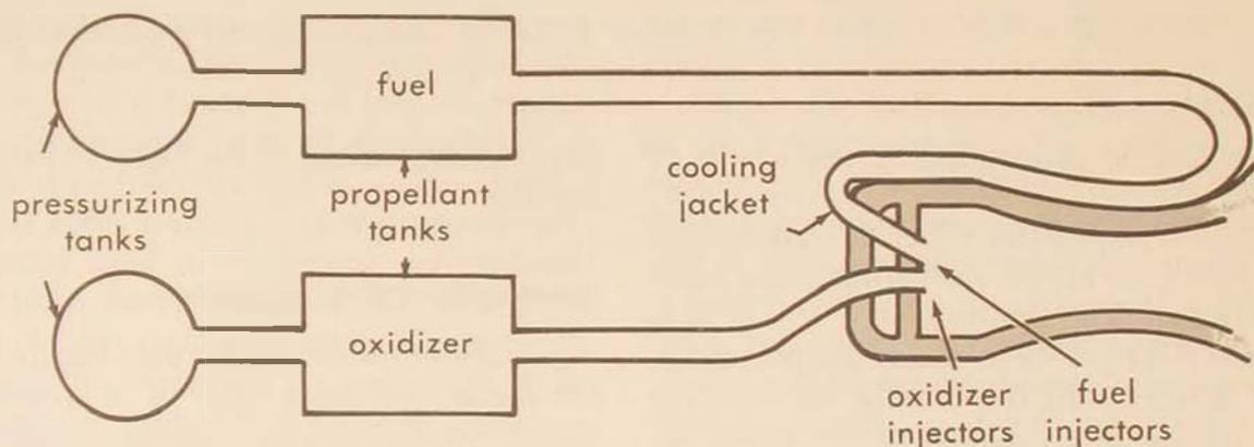
Figure 7. Pressure-fed bipropellant system
