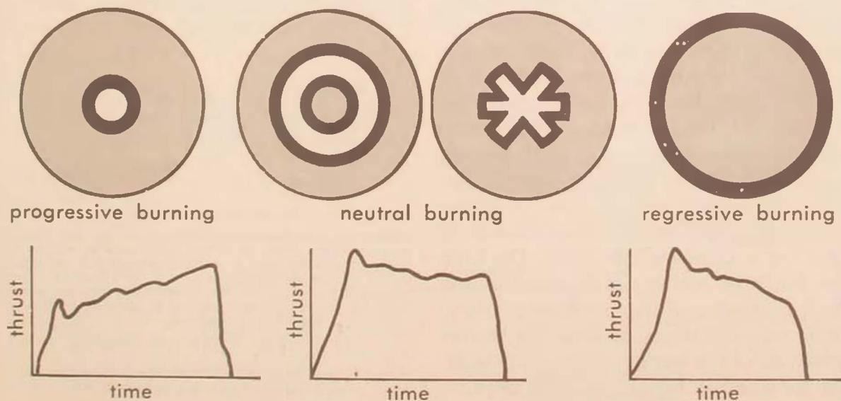
ing surface. With progressive burning, the area of propellant under combustion increases with time. This increasing propellant consumption rate provides a continually increasing mass of exhaust products and a corresponding increase in thrust. In neutral burning, by special design of the core, the area under combustion is held relatively constant, and the thrust from this effect is constant. With regressive burning, combustion area continually decreases, with a resulting decrease in thrust.
