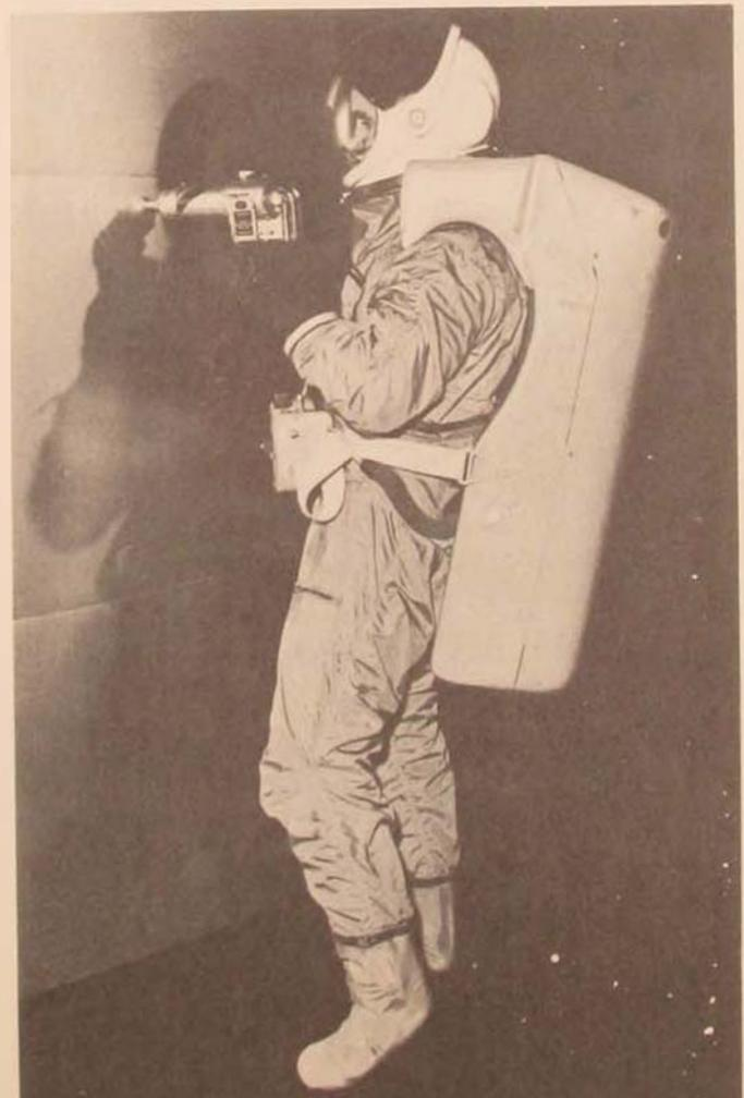
*Representation of astronaut using minimum-reaction space tool*
