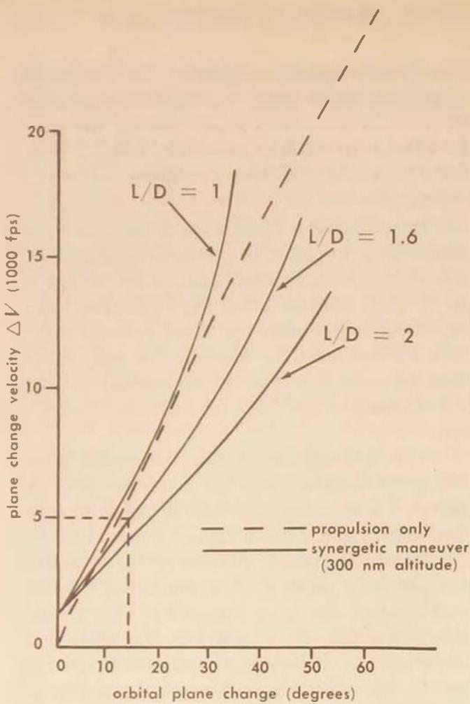
Figure 6. Comparison of plane change velocity requirements
