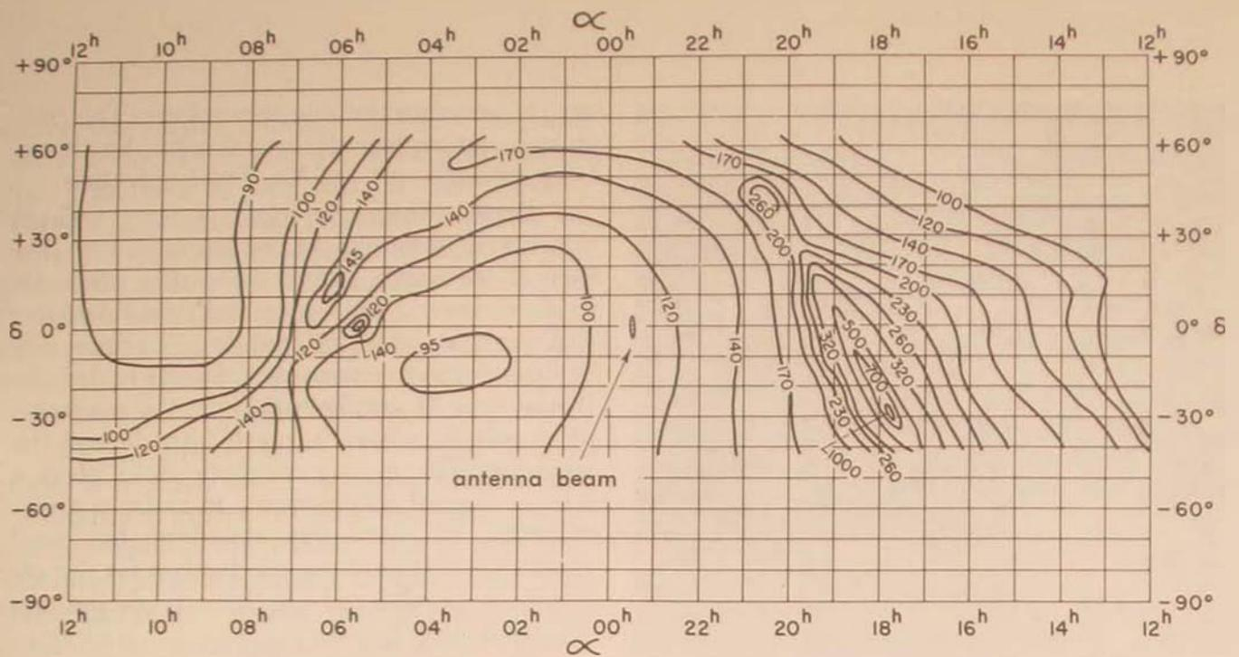
The solar photosphere was photographed in Hydrogen Alpha during a period of solar activity by astronomers at Sacramento Peak Observatory, New Mexico. The white areas are plages, and the darker spots are solar flares. . . . Plots such as this are made, at various frequencies, of the intensity of radio noise emanating from large general areas of space.
