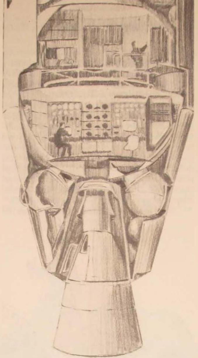
Figure 3. The Medium Orbital Research Laboratory
