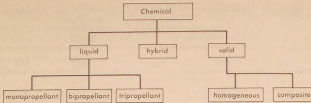
Figure 2. Classification of chemical propulsion systems
