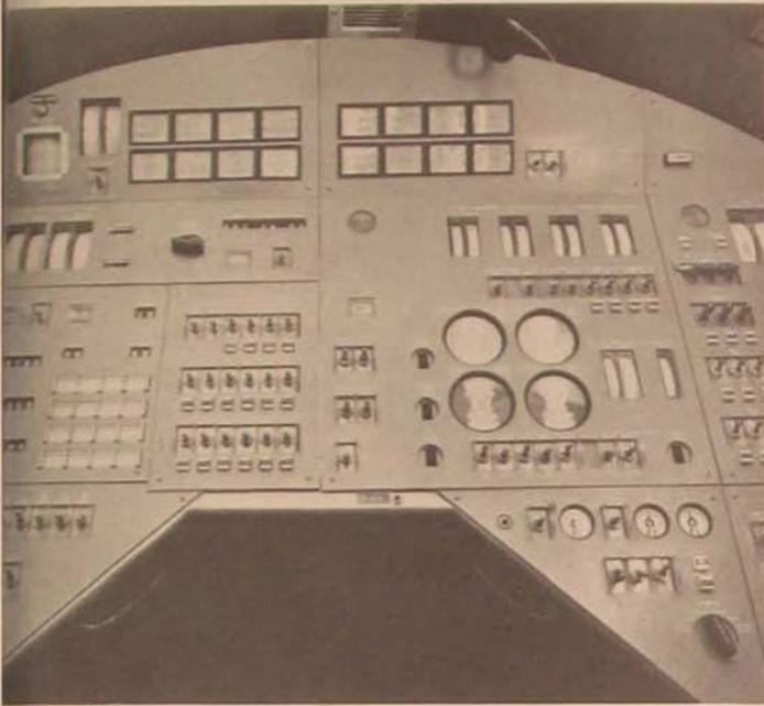
by an analog computer tie-in between the attitude stick in the excursion module and the projector. When the pilot pitched the excursion vehicle away from the lunar surface, the horizon disappeared and more stars came into view.
