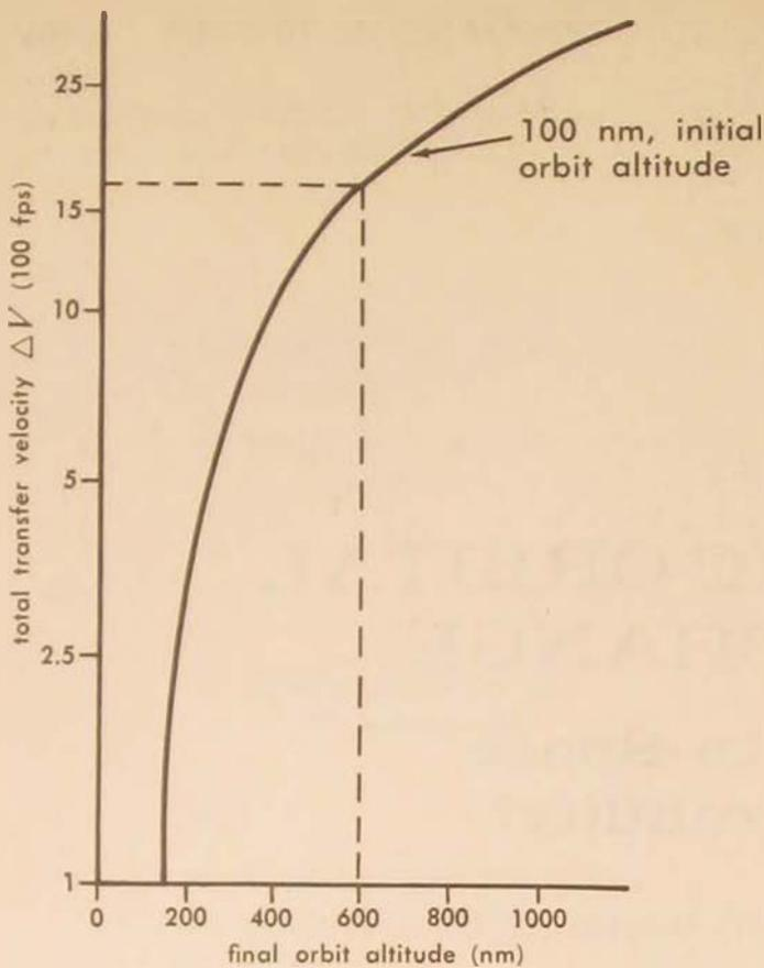
Figure 2. Hohmann transfer velocity requirements
