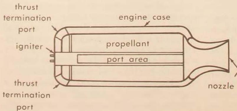
Figure 9. Typical solid-rocket engine
