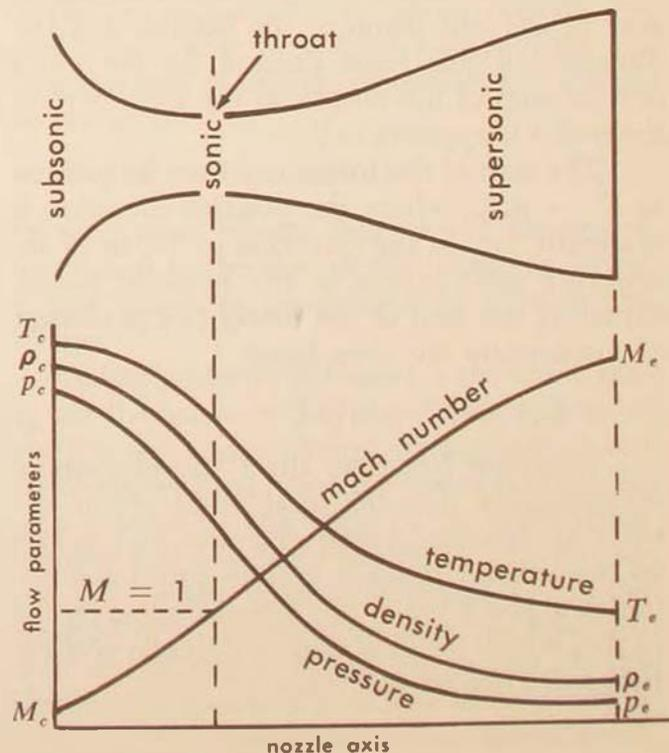
The momentum thrust term is by far the predominant one. It is dependent upon (1) the particular exhaust gas, or mixture of gases, (2) the combustion chamber pressure,  $p_c$ , and (3) the geometry of the nozzle. Thus it is independent of the environment in which the rocket operates and is a function only of the design of the rocket engine.
