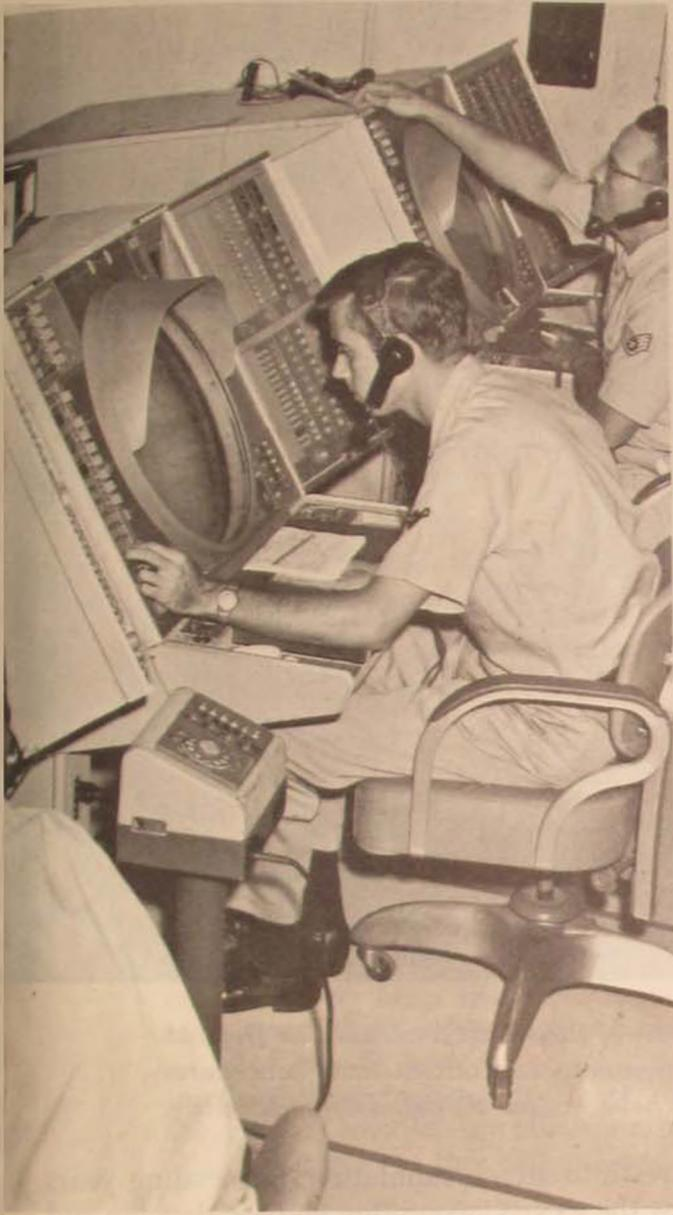
imulation team members direct their interceptors toward approaching enemy aircraft during a simulated mission. By using switch actions, the "intercept pilots" are able to guide their aircraft to the target.
