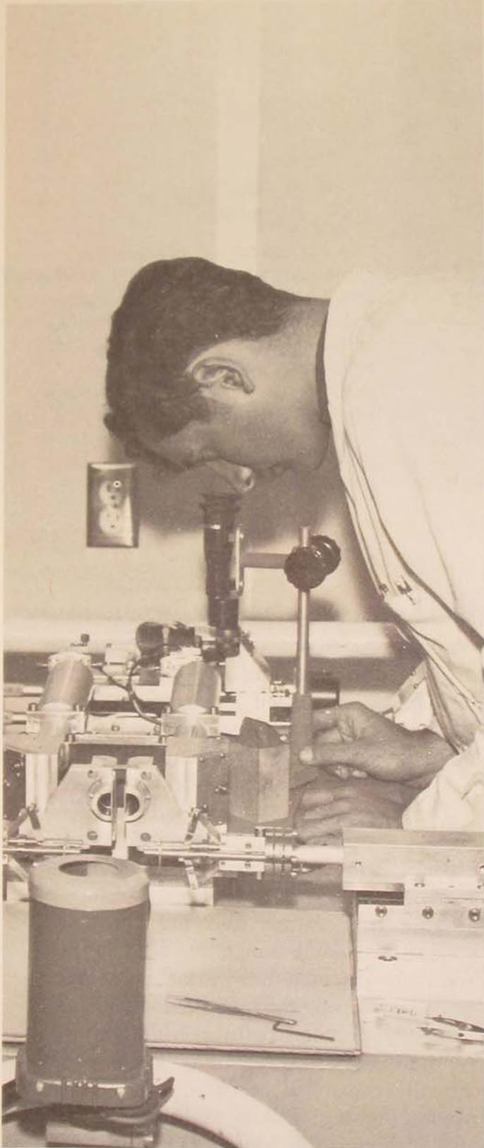
*A Stress/Strain Analyzer optically measures filament elongation to obtain a comparison of the stress versus strain for very-high-modulus monofilaments such as boron, sapphire, and graphite.*
