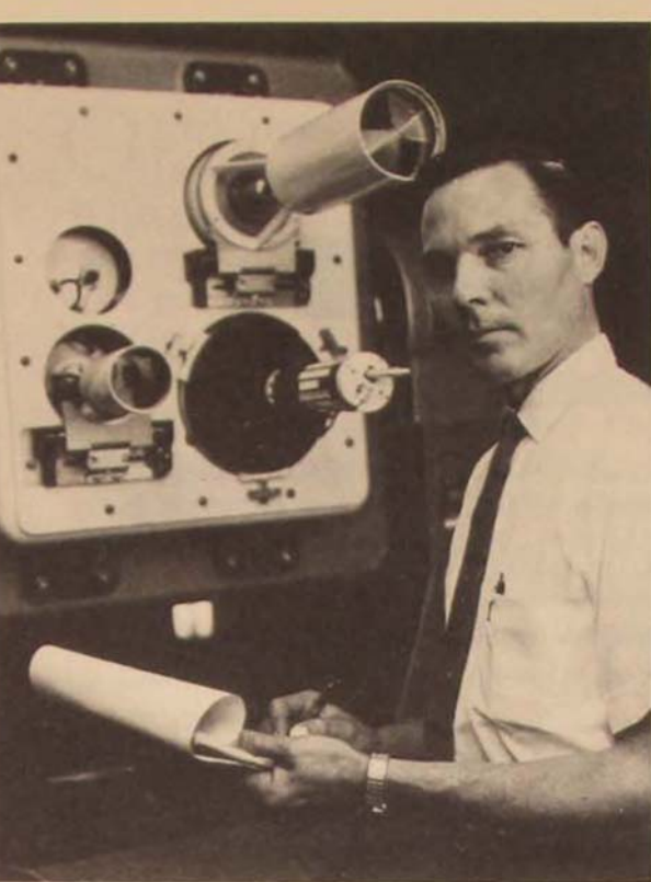
A unique dual laser system is employed in geodetic satellite studies by scientists at the Air Force Cambridge Research Laboratories. A ranging short-pulse laser is housed in the lower left side of the mount; a long-pulse photographic laser is shown (upper right), as well as high-voltage and receiver components.
