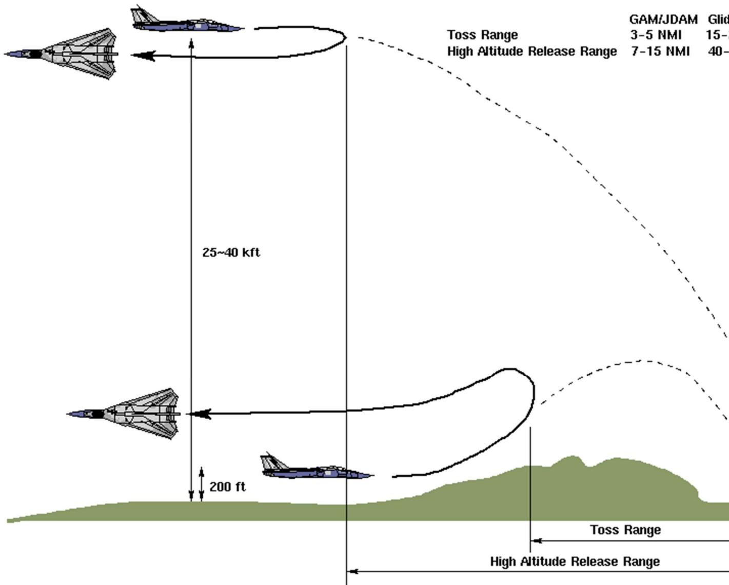
**FIG.10 DELIVERY PROFILES FOR GPS/INERTIAL GUIDED WEAPONS**
