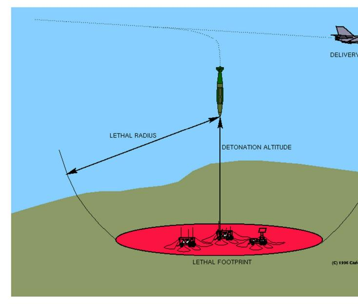
FIG.7 LETHAL FOOTPRINT OF LOW FREQUENCY E- BOMB IN RELATION TO ALTITU
