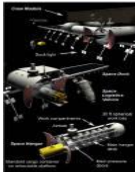
Figure 6. Notional Space Logistics Base consisting of twin, opposite-facing, space hangars, with an upper crew module and a lower space dock. In the top illustration, an SLV tug is maneuvering a cargo module while the second stage of a near-term RLV off-loads cargo. A passenger spaceplane is entering the nearest hangar. In the center illustration, an SLV tug positions a satellite at the entrance to the space hangar. The bottom illustration shows a cut-away view of the space hangar.
