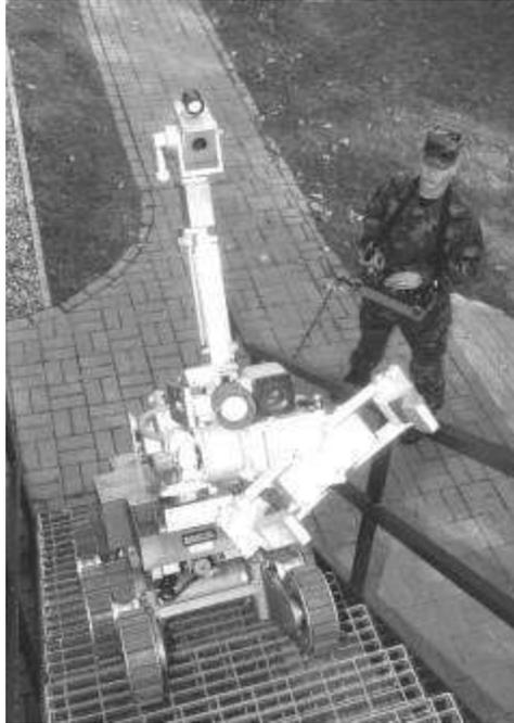
MK III RONS Robotics all-terrain, tracked vehicle with manipulator arm and TV cameras.
