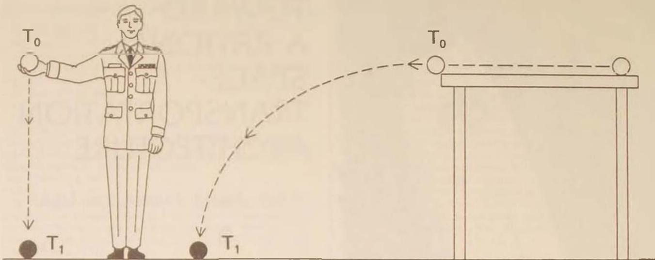
Figure 1. The time of fall for two objects dropped from equal heights is the same, regardless of forward velocity.
