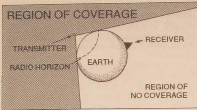
Figure 4. Direct Line-of-Sight Limitations of a Low-Altitude Transmitter. From AU-18, *Space Handbook*, ed. Lt Col Curtis D. Cochran, Lt Col Dennis M. Gorman, and Maj Joseph D. Dumoulin (Maxwell AFB, Ala.: Air University Press, January 1985), 7-5.
