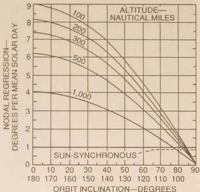
Figure 8. Nodal Regression Rate Per Day for Circular Orbits and Sun-Synchronous Altitudes. From AU-18, *Space Handbook*, ed. Lt Col Curtis D. Cochran, Lt Col Dennis M. Gorman, and Maj Joseph D. Dumoulin (Maxwell AFB, Ala.: Air University Press, January 1985), 2-43.
