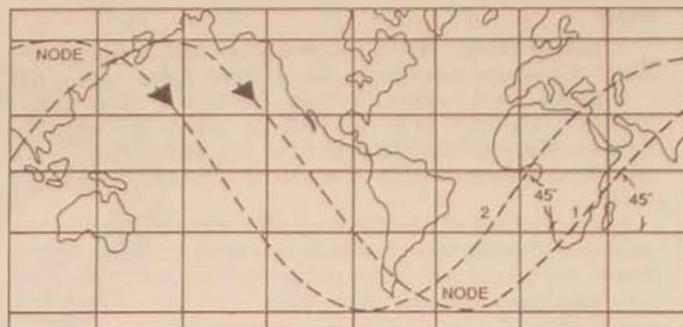
Figure 10. Two Equally Inclined Noncoplanar Orbits. Adapted from AU-18, *Space Handbook*, ed. Lt Col Curtis D. Cochran, Lt Col Dennis M. Gorman, and Maj Joseph D. Dumoulin (Maxwell AFB, Ala.: Air University Press, January 1985), 2–33.
