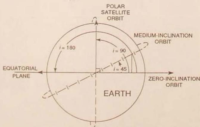
Figure 3. Measuring Inclination
