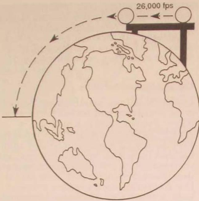
Figure 2. An object traveling 26,000 feet per second will fall toward the earth's surface along a trajectory that matches the contour of the earth.
