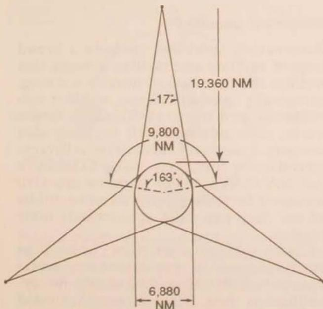
Figure 5. Concept of Three Communications Satellites in 24-Hour Equatorial Orbit, Showing Geometrical Relationships in the Equatorial Plane. From AU-18, *Space Handbook*, ed. Lt Col Curtis D. Cochran, Lt Col Dennis M. Gorman, and Maj Joseph D. Dumoulin (Maxwell AFB, Ala.: Air University Press, January 1985), 7-4.
