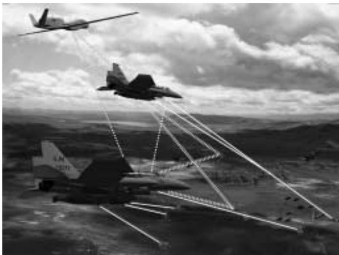
**Figure 4. The Final Link.** Data from the two strike aircraft, working in cooperation, is burst data-linked to a “traditional” ISR platform, the RQ-4 Global Hawk, providing an extension to the UAV’s own sensor array.
