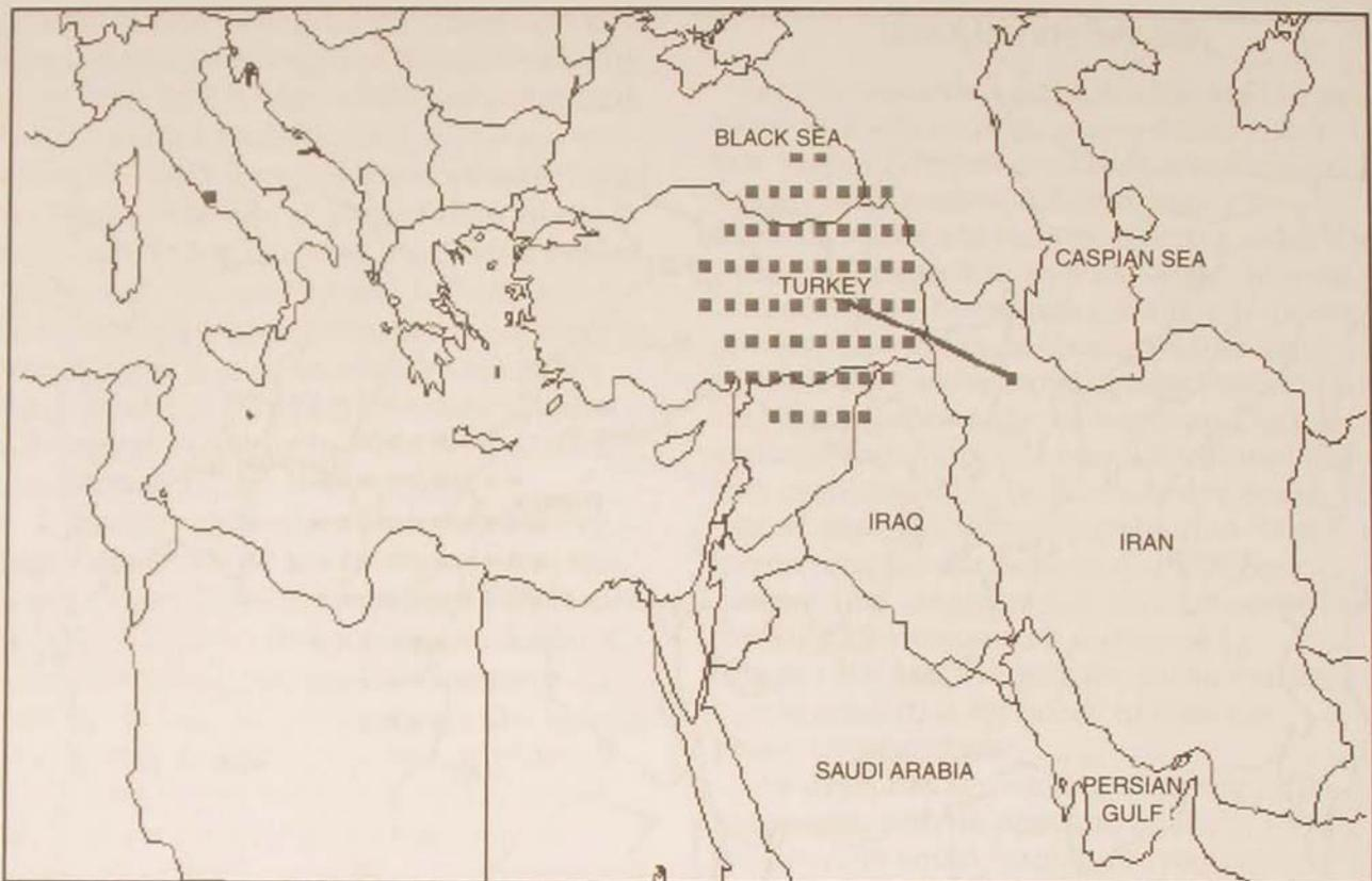
**Figure 7. Ascent-phase operational area, assuming launch of a 3.5 km/sec interceptor 80 seconds after detection of the IRBM target and interception of target 270 seconds later (two minutes after IRBM burnout)**
