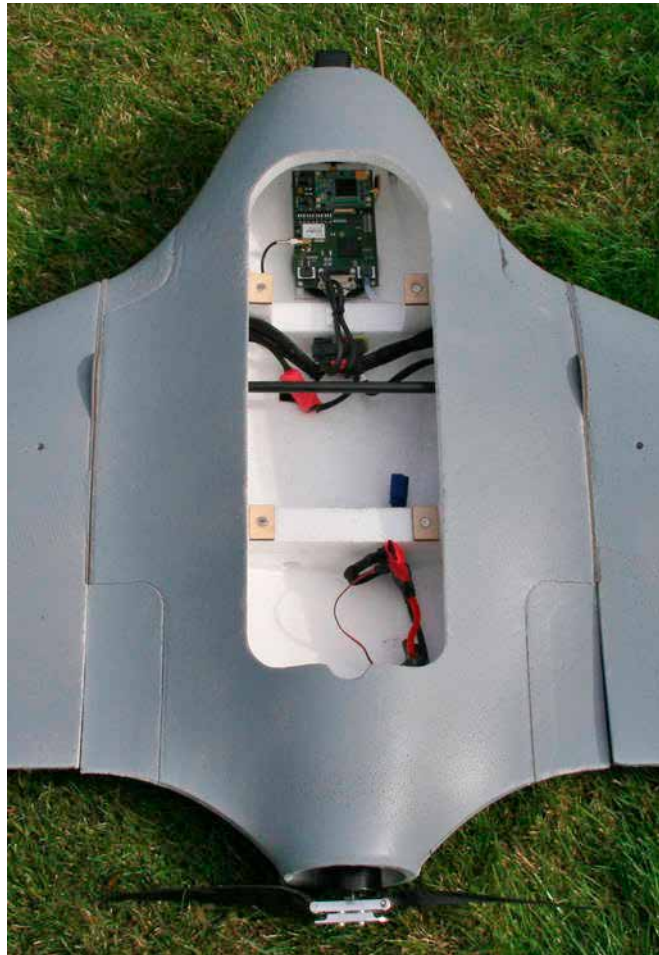
Figure 2. X8 Flying Wing internal storage
