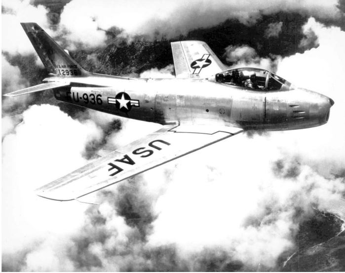
Fig. 15. The North American F-86 Sabre battled Communist MiG-15s for air superiority over “MiG Alley” in the Korean War. The wraparound glass cockpit provided excellent visibility. Courtesy of AFHF.
