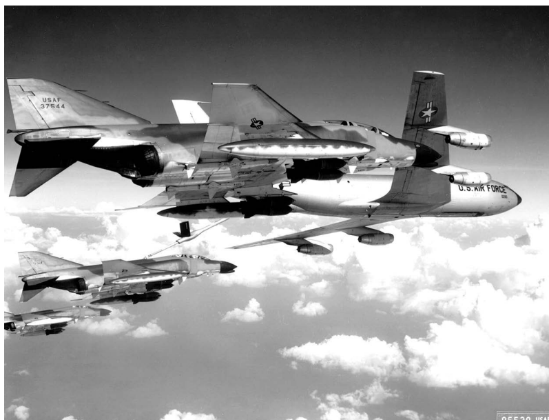
Fig. 19. McDonnell-Douglas F-4 Phantoms being refueled by a Boeing KC-135 enroute to striking targets in North Vietnam. Each Phantom is carrying two external fuel tanks, four Mark 82 bombs, and three AIM-9 Sidewinder air-to-air missiles. Courtesy of AFHF.
