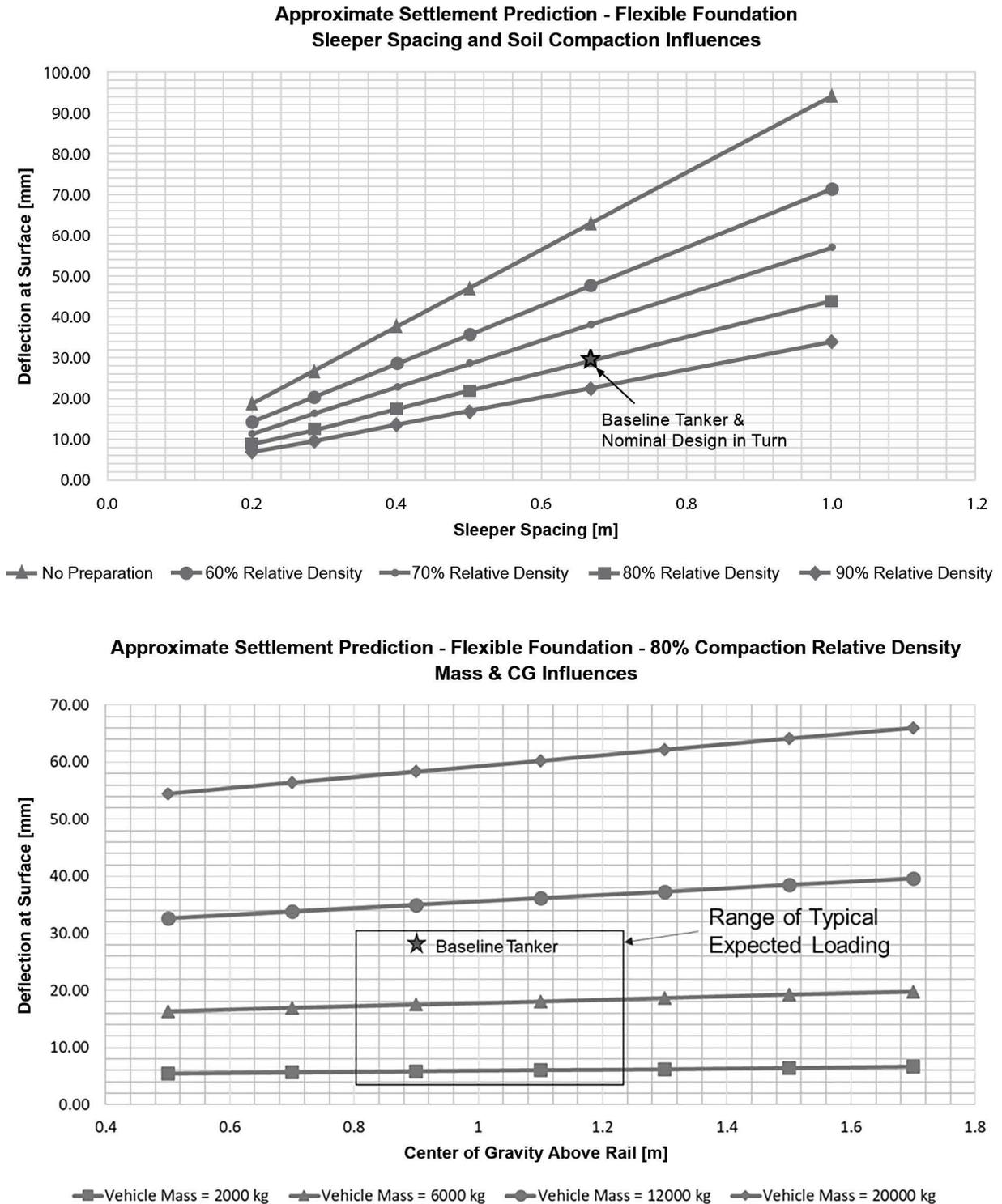
Figure 12.4. Geotechnical analysis summary plots for peak dynamic loading. [Credit: Northrop Grumman]
