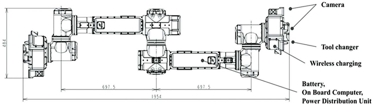
Figure 8.1. The Inchworm robot. [Credit: GITAI]
