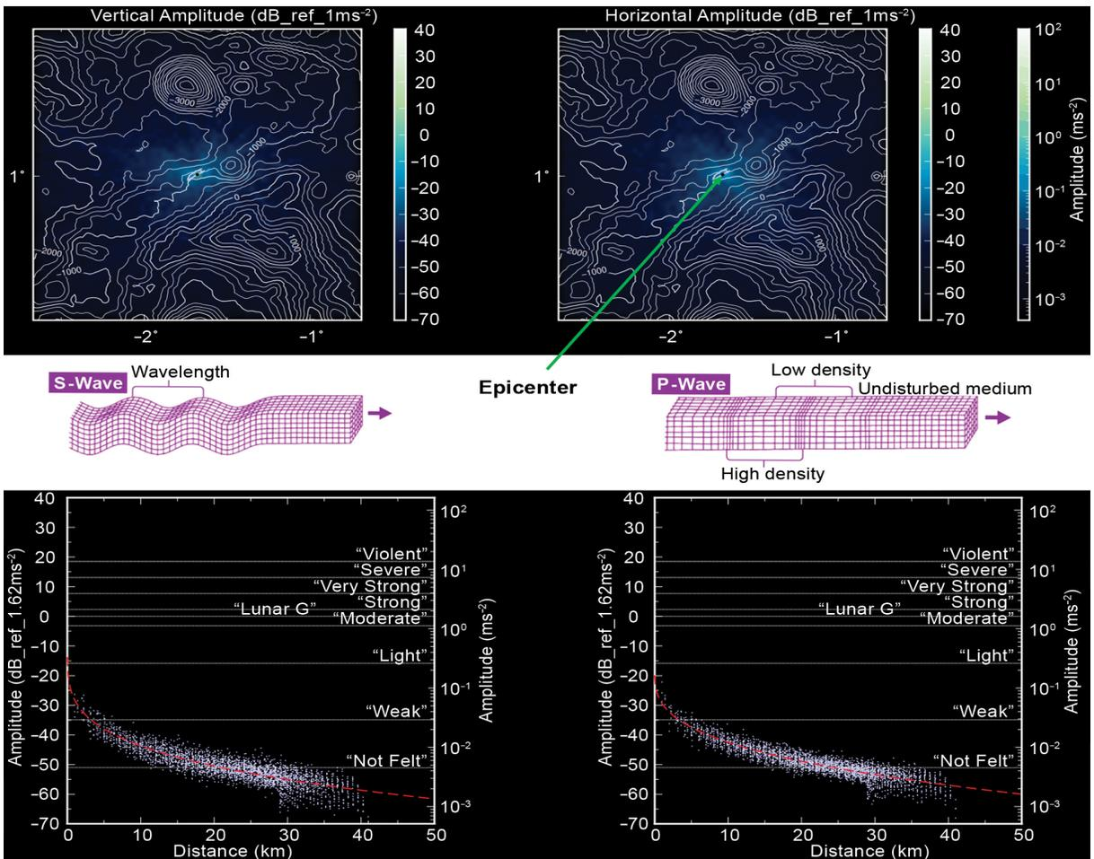
**Figure 10.2.** (Top) Heat map of S- and P-wave amplitude as a function of distance from the epicenter of crash anomaly. (Bottom) Amplitude of S- and P-waves as a function of distance from the epicenter of crash anomaly. [Credit: Honeybee Robotics]
