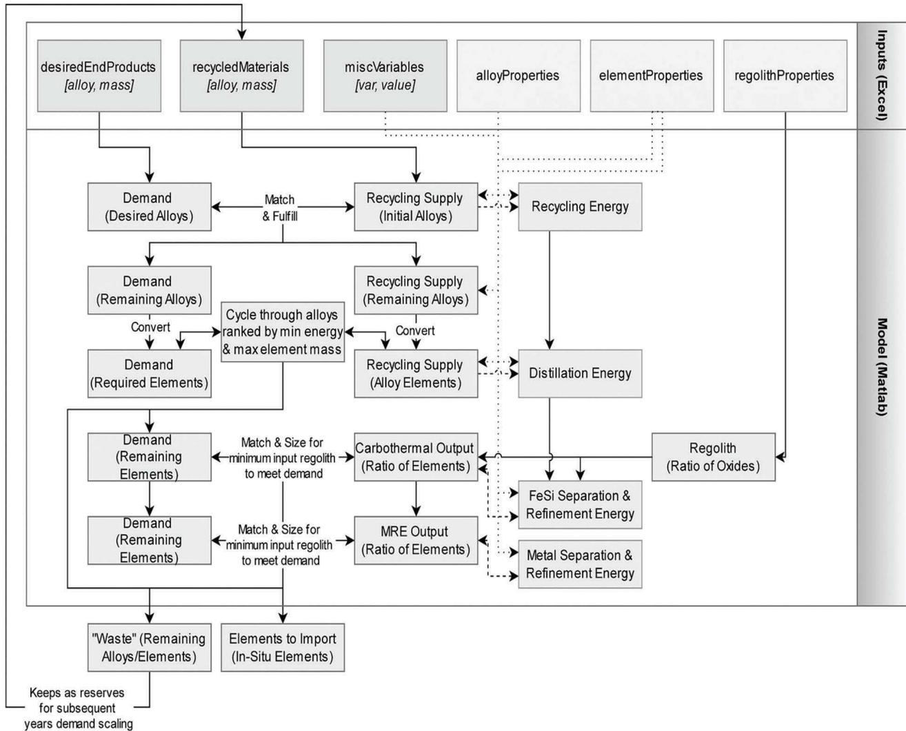
**Figure 6.4.** Metal framework energy-mass model. [Credit: CisLunar Industries]
