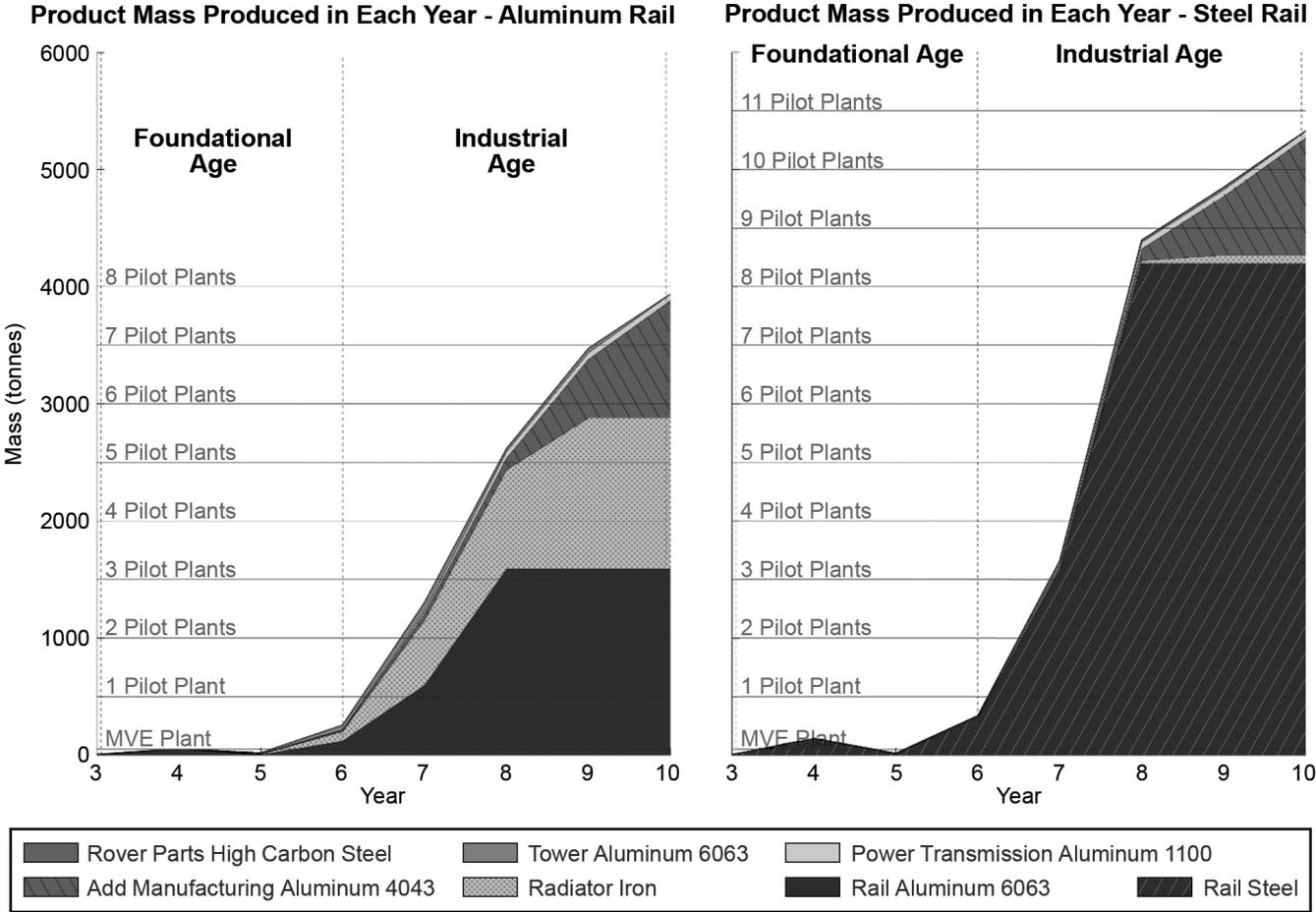
Figure 6.6. Foundry product production by mass versus year; (left) aluminum rail and (right) steel rail.
