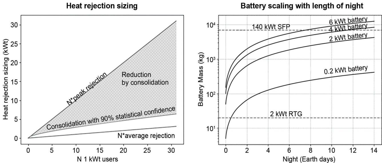
**Figure 11.2.** (Left) Benefit of consolidation. Plot shown with 1  $\text{kW}_t$  users with a ten-to-one peak to average duty cycle. Consolidation line is the expected peak sum with 90 percent confidence using a one-tailed student t-test with a peak of two standard deviations from average. (Right) Battery mass as a function of lunar night length. Masses of surface fission power<sup>7</sup> and a radioisotope thermoelectric generator are shown for comparison. [Credit: Honeybee Robotics]
