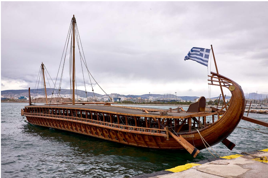
Reconstruction of an Athenian trireme, which featured rowers on three separate levels of the vessel. Photo courtesy of George E. Koronaios (CC BY-SA 4.0).
