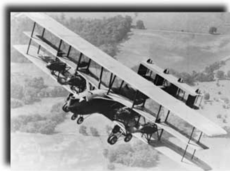
The Barling Bomber was a six-engined behemoth capable of carrying a 10,000-pound payload. However, it did not even have enough power to fly over the Appalachian Mountains.
