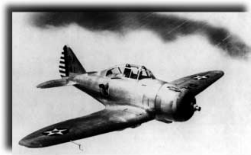
The Seversky P-35, a forerunner of the Republic P-47, was the first single-seat, all-metal pursuit plane with retractable landing gear and enclosed cockpit when it entered Air Corps service in 1937.
