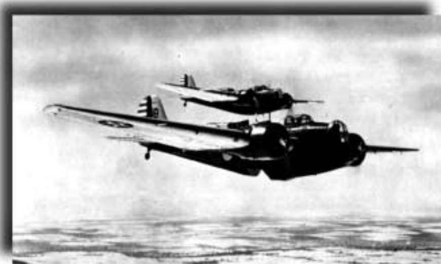
The Martin B-10 represented a new generation of bombers. It featured enclosed cockpits, a power-operated turret, and retractable landing gear.
