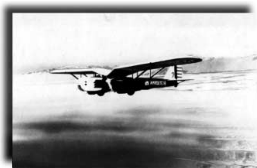
The Douglas B-7, designed as a fast day bomber, had fabric-covered wings, an all-metal fuselage, and hydraulically operated retractable landing gear. It flew airmail over the Salt Lake City–Oakland route in early 1934.
