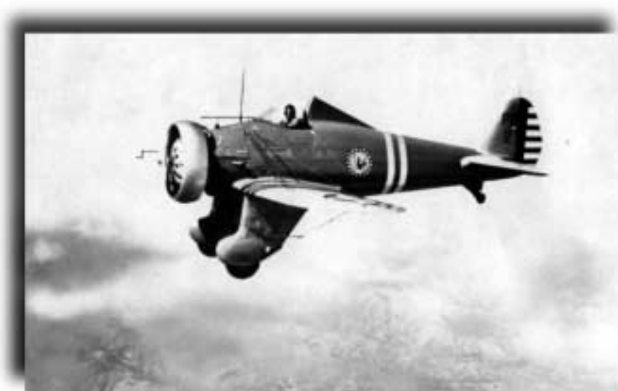
Designed to meet the increasing performance of the new bombers, the Boeing P-26 Peashooter was the first all-metal monoplane fighter built for the Army Air Corps.
