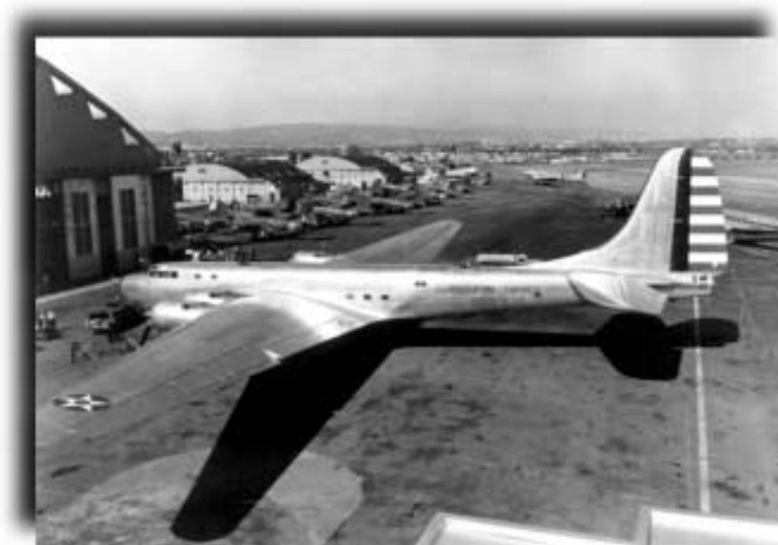
The Douglas XB-19, which first flew in 1941. With a wingspan of 212 feet, a 132-foot fuselage, and a rudder 42 feet high, it dwarfed other aircraft of its day.
