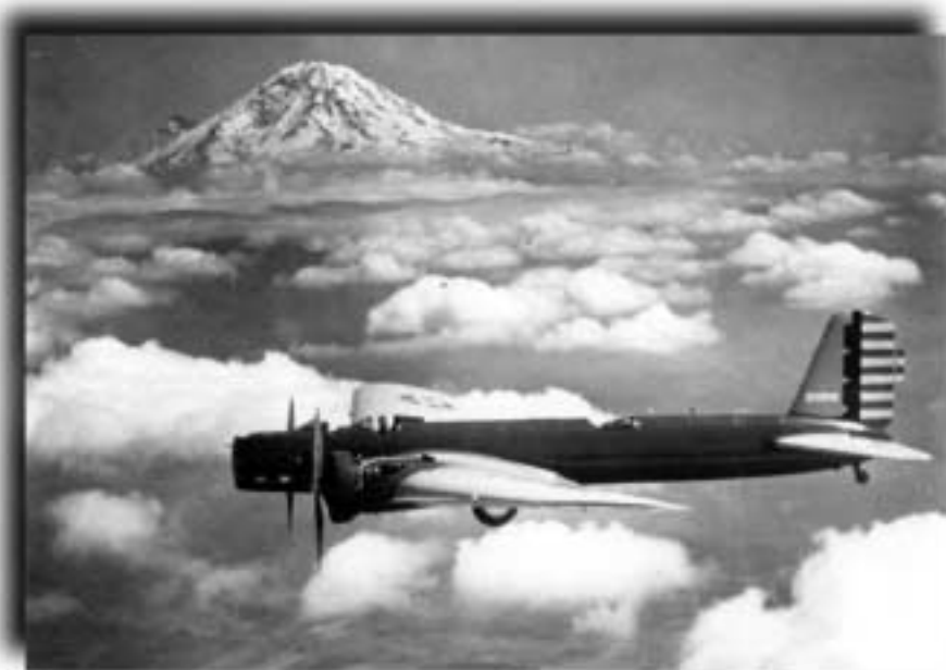
The Boeing B-9 bomber, a low-wing, all-metal monoplane, was introduced in the 1930s. Although it still had open cockpits, it had the “big bomber” look that raised the hopes of airmen who believed in strategic bombardment.
