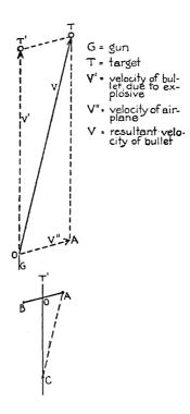
Figure 6. Principle of the Wind-Vane Sight
