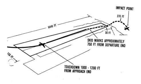
**Figure 74. Touchdown, no braking, braking too late, crash.** (Reprinted with permission from Sharon O'Malley Burg.)
