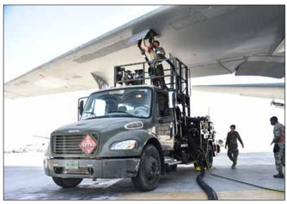
US forces enjoyed access to modern airfields with enhanced, integrated logistics systems to support sustained (and often intense) flying operation. Here a ground crew pumps a portion of the more than 500,000 gallons of aviation fuel processed daily at the fuel bladder farm at Al Dhafra Air Base, United Arab Emirates.
