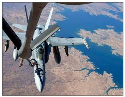
A US Navy F-18 refuels from a KC-135 during a strike mission against ISIS forces in 2014. Note the "basket" signifying the probe and drogue refueling system used by naval and allied aircraft. The KC-135 must be configured on the ground for either boom or drogue missions, thus limiting its flexibility once airborne.
