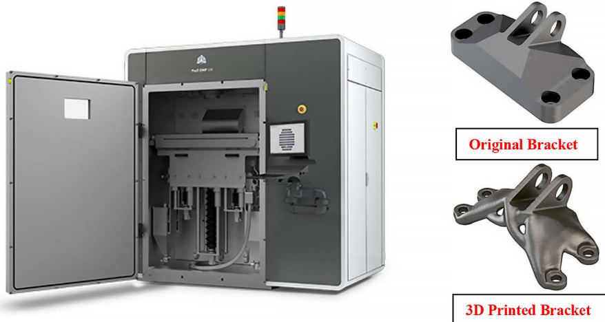
Figure 5. ProX DMP 320 3-D Printer 93 and Aircraft Brackets 94
