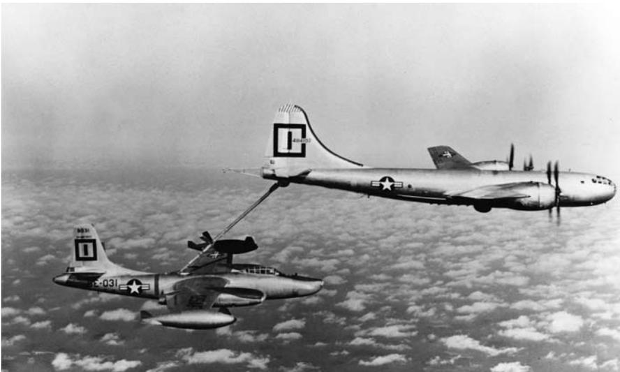
Figure 7. KB-29 refueling B-45 after World War II, developed to extend the reach of jets to ultimately reach a Global Strike Capability.
