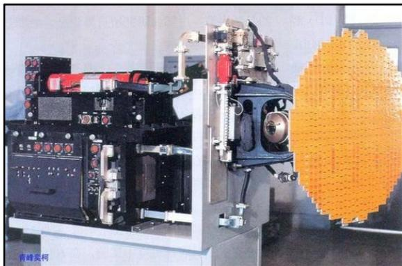
LETRI continues to be a leading developer of airborne radar systems for the Chinese military as well as civilian end-users. In 2018 LETRI displayed an X-band AESA radar at the Zhuhai Airshow. Accompanying exhibits indicated that the radar is capable of detecting fighters 170 km away and can track 15 targets at the same time.<sup>88</sup>
