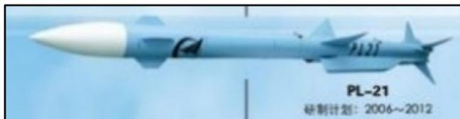
The PL-21 (also referred to as the PL-XX, since the missile's actual designation, or even its existence, cannot be confirmed) is said to be a ramjet-powered active radar-homing very long-range air-to-air missile
