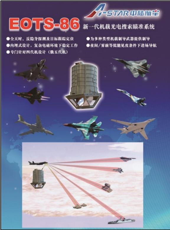
An EOTS system similar to that used on the F-35 is said to be under development by the Beijing “A-Star” Science and Technology Co. [北京中陆航星科技有限公司], profiled in a later section. Beijing “A-Star” has shown its own EOTS-86 system, which the company claims can detect stealthy aircraft such as the B-2 bomber from over 100km away.
