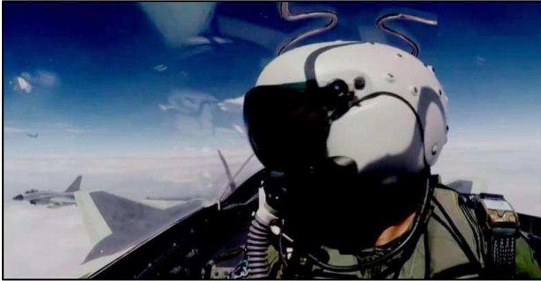
the helmet does not incorporate night vision sensors.<sup>194</sup> The helmet system can be used to lock and fire PL-9 or PL-10 AAMs.
