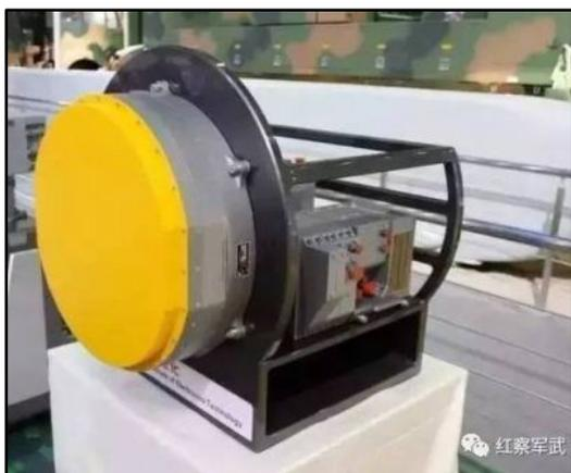
The KLJ-7A or Type 14789 is an X-band airborne fire-control radar produced by the CETC 14<sup>th</sup> Research Institute. China is upgrading JF-17 fighter aircraft it co-produced with Pakistan with new radars, and the KLJ-7A would "tremendously extend the fighter's detection range."<sup>184</sup>
