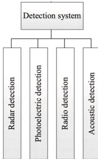
Figure 4: Categories of LSS detection technologies described by PRC defense engineers<sup>46</sup>
