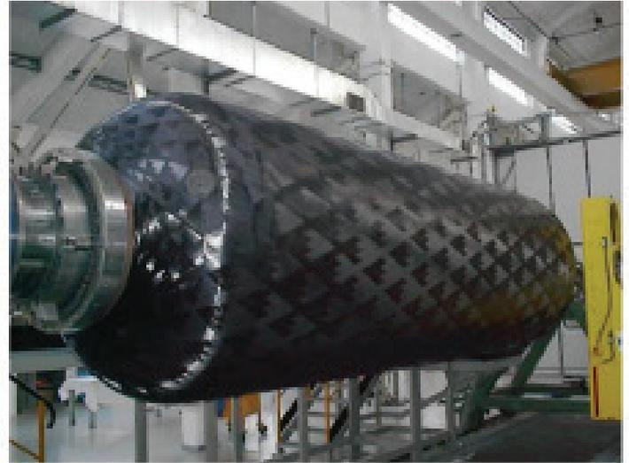
*Examples of missile bodies made by filament winding*
