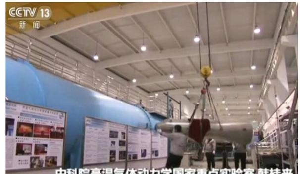
Reentry vehicle test body being lifted into a hypersonic wind tunnel (FL22)
