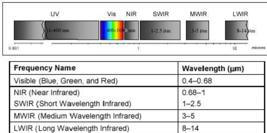
**Figure 2 Wavelength Groupings for HSI Sensors**
