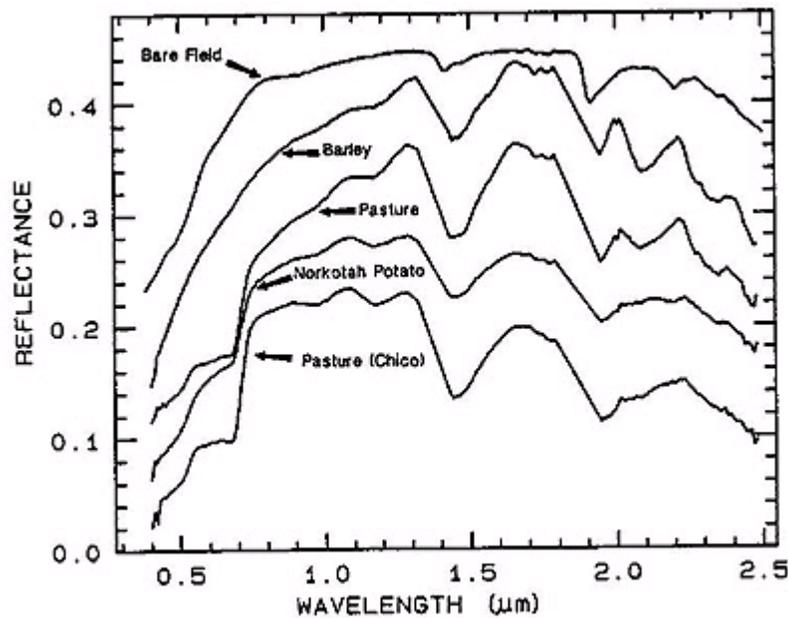
**Figure 1: Spectral Signatures Constructed From AVIRIS Sensor**
