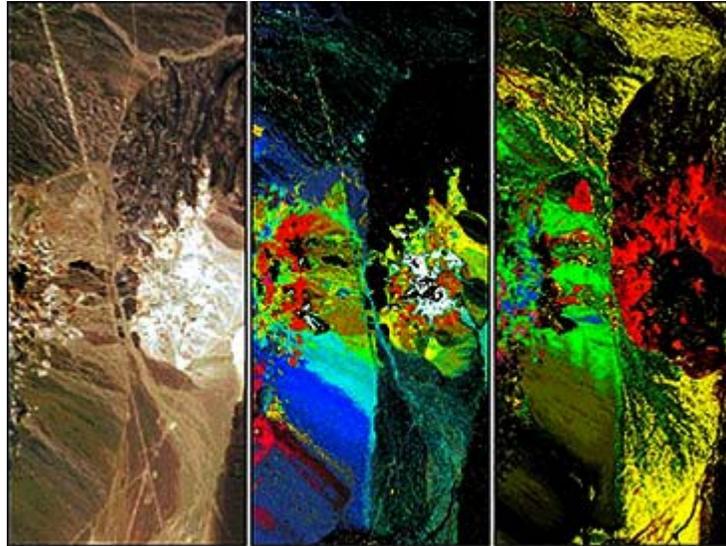
**Figure 4: Comparison of Two False-Color HSI Images with Natural Color Photo<sup>13</sup>**
