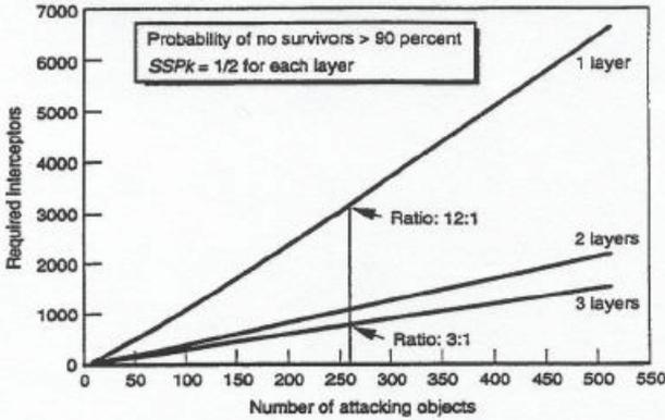
**Figure 4. Layering Reduces Sensitivity to Attack Size<sup>42</sup>**
