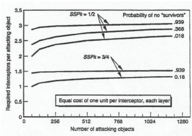
**Figure 7. Cost per Attacking Object is Sensitive to Probability of Kill ( $P_k$ )<sup>48</sup>**
