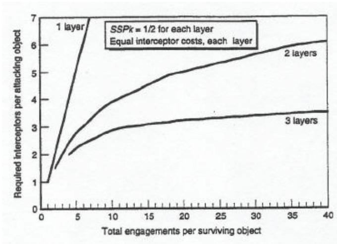
**Figure 6. Layering Reduces Cost per Attacking Warhead<sup>45</sup>**
