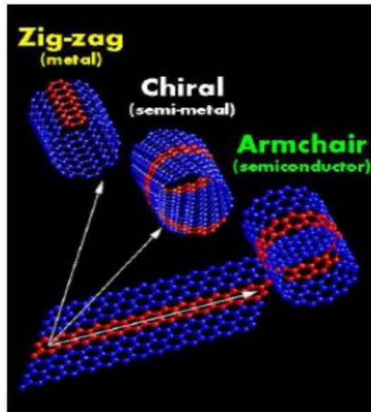
Figure 3: Three Forms of Carbon Nanotubes Based on Chirality 21
