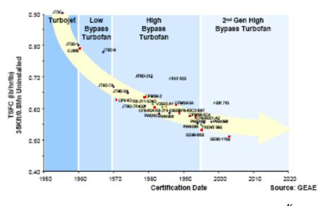
Figure 11: Evolution of Gas-Turbine Fuel Efficiency<sup>46</sup> (Source: GE Aircraft Engines, through Scientific Advisory Board)
