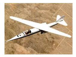
Figure 9: NASA AD-1 Oblique Wing Demonstrator<sup>40</sup> (Source: NASA Dryden Flight Research Center)
