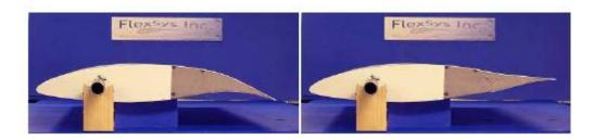
Figure 8: Mission Adaptive Compliant Wing (made for AFRL by FlexSys Inc)<sup>38</sup>
