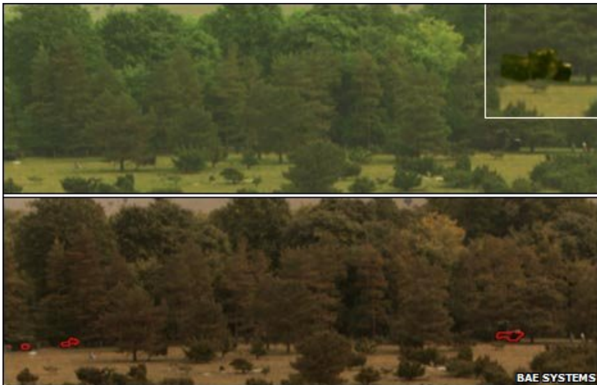
Figure 4. Hyperspectral techniques enable the sensor to identify the green vehicle in the trees, they are shown in red in the lower image. Obtained from the internet, http://www.bbc.co.uk/news/10175960
