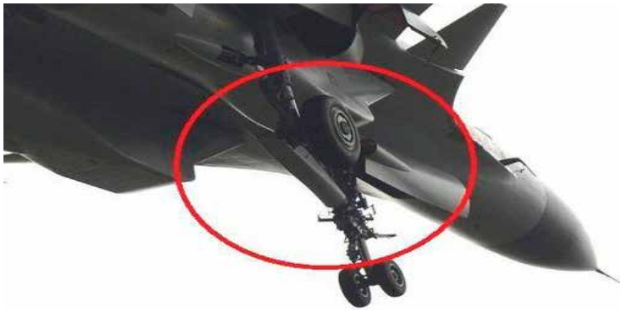
Figure 2. New capability. Shenyang J-15 Flanker-X-2 carrier-based multirole fighter with a catapult launch bar (CATOBAR) on its front wheel, which is used to couple the aircraft to the catapult during takeoff. Given this new development, it is presumed that China's third aircraft carrier, planned to be built at the Jiangnan Shipyard, will employ a catapult system.
