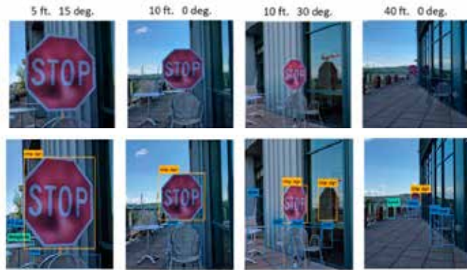
Figure 2. (Top) Adversarial 2D camouflage to a stop sign imitating wear and tear, using a convolutional neural network—a class of deep, feed-forward artificial neural networks, most commonly applied to analyzing visual imagery—on the Laboratory for Intelligent and Safe Automobiles road-signs database, achieves 100-percent success classifying each of these as 45-mph-speed signs. (Kevin Eykholt et al., “Robust Physical-World Attacks on Deep Learning Visual Classification” (paper, 2018 Conference on Computer Vision and Pattern Recognition, Salt Lake City, UT, 18–22 June 2018), https://arxiv.org/pdf/1707.08945.pdf .) (Bottom) For a detector followed by a classifier—a mapping from unlabeled instances to discrete classes—achieves 100-percent failure, correctly identifying these as stop signs every time. (Jiajun Lu et al., “Standard Detectors Aren’t (Currently) Fooled by Physical Adversarial Stop Signs,” 26 October 2017, https://arxiv.org/pdf/1710.03337.pdf .)
