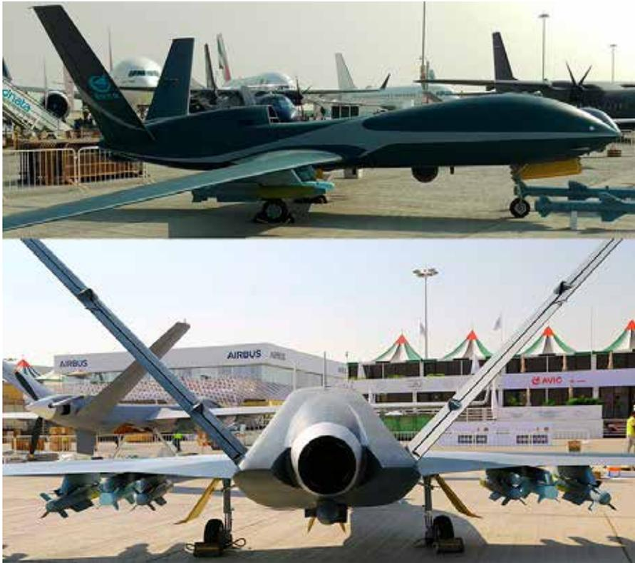
**Figure 2.** The Cloud Shadow high-altitude, long-endurance (HALE) unmanned aerial system. This UAS was unveiled at the Airshow China 2016 exhibition held in Zhuhai, China.
